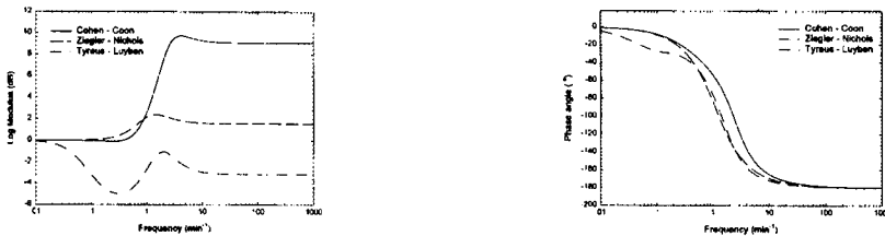
Figure 11: Closed loop Bode plot of the TOPIR process with \tau = 1, \zeta = 1 controlled with PID control using Cohen-Coon, Ziegler-Nichols, and Tyreus-Luyben control constants.
