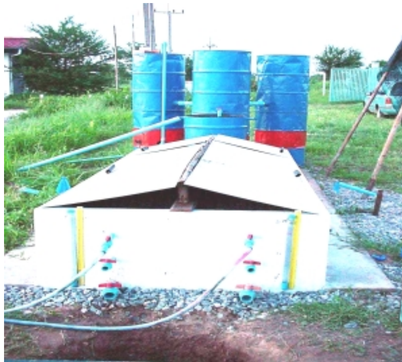
Figure 3-3. Front view of pilot-scale rock-bed filtration units.
