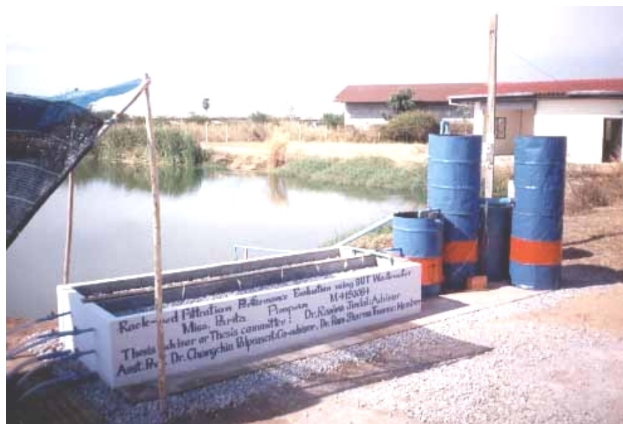
Figure 3-4. Side view of pilot-scale rock-bed filtration units.
