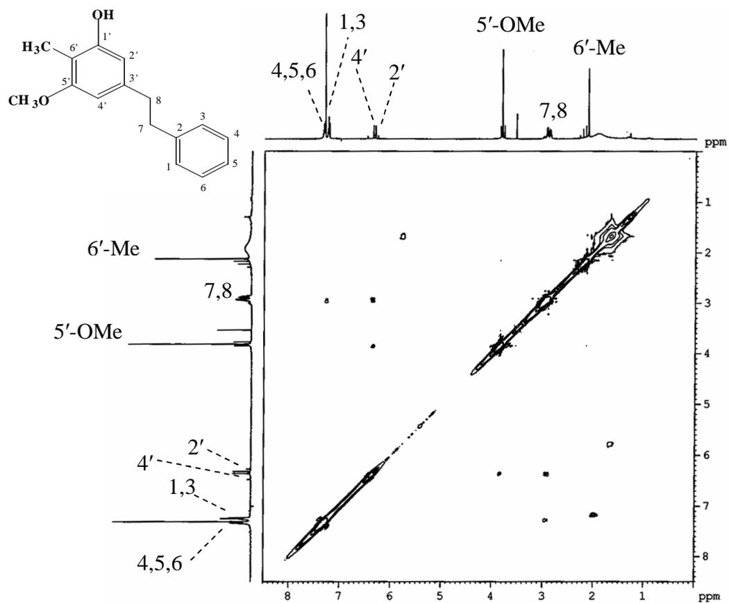
Figure 3.9 NOESY spectrum of compound III
