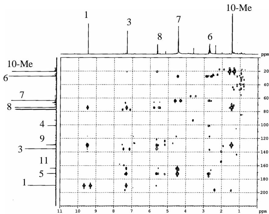
Figure 11.7 HMBC spectrum of compound XI
