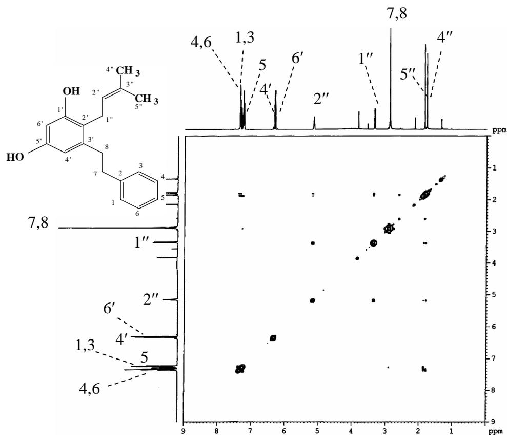
Figure 6.8  $^1\text{H}$ ,  $^1\text{H}$ -COSY spectrum of compound VI
