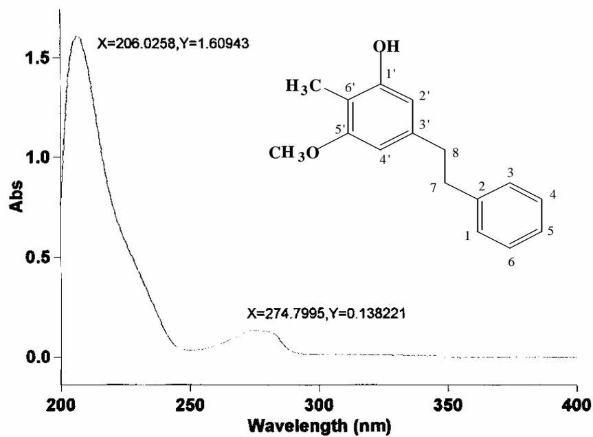
Figure 3.3 UV-Vis spectrum of compound III
