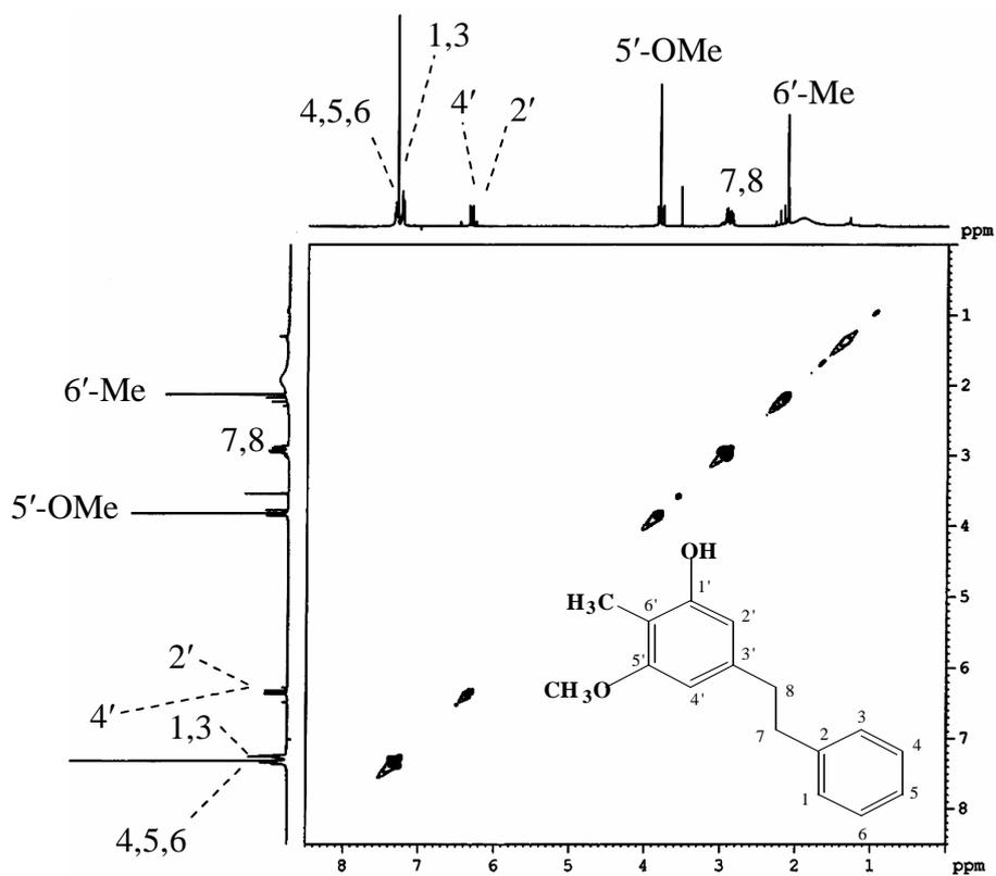
Figure 3.8 <sup>1</sup>H, <sup>1</sup>H-COSY spectrum of compound III
