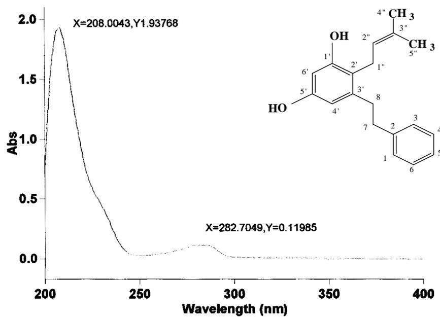
Figure 6.3 UV-Vis spectrum of compound VI
