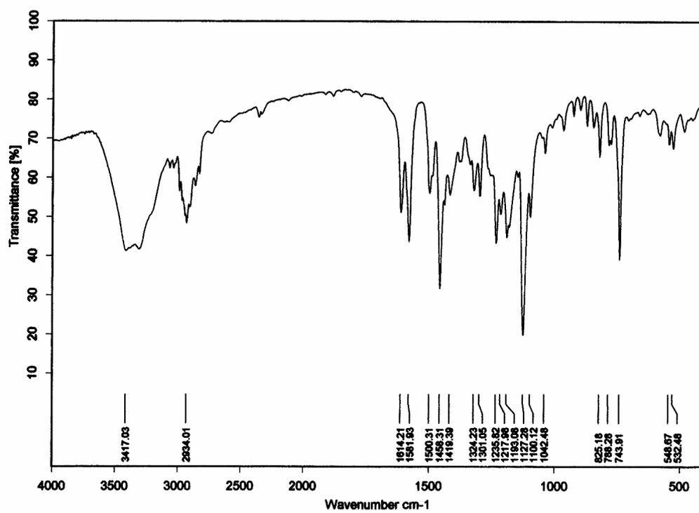
Figure 2.2 IR spectrum of compound II
