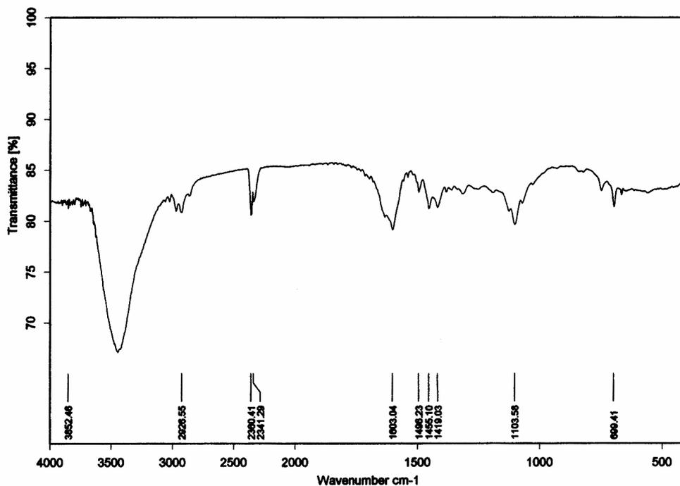
Figure 4.1 IR spectrum of compound IV
