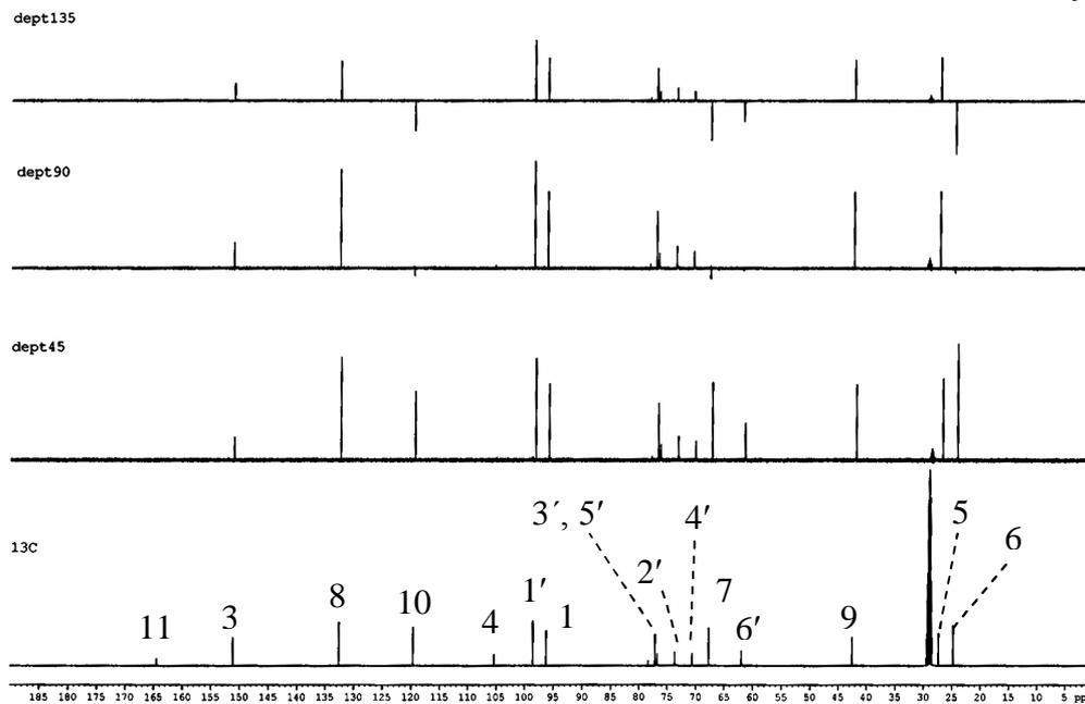
**Figure 12.5**  $^{13}\text{C}$ -NMR and DEPT spectra of compound **XII** in acetone- $d_6$
