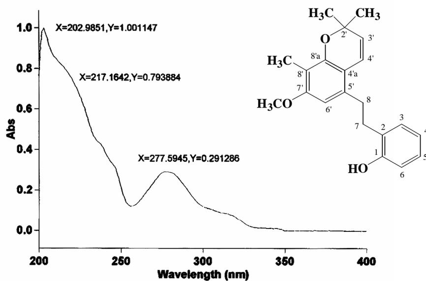
Figure 1.3 UV-Vis spectrum of compound I
