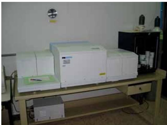
**Figure 3.6** FTIR spectrometer Perkin-Elmer model: spectrum GX.
