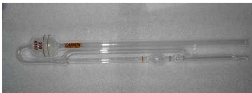
**Figure 3.4** A Cannon Ubbelohde capillary viscometer No 150.
