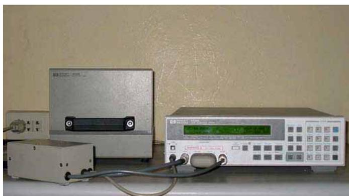
**Figure 3.9** Hewlett-Packard 4339B high resistance meter.
