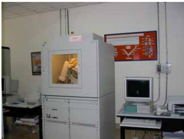
**Figure 3.7** Bruker, model D5005 X-ray diffractometer with Ni-filtered Cu  $K_{\alpha}$
