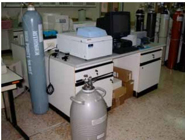
**Figure 3.8** PerkinElmer PYRIS (Diamond) Differential Scanning Calorimeters (DSC).
