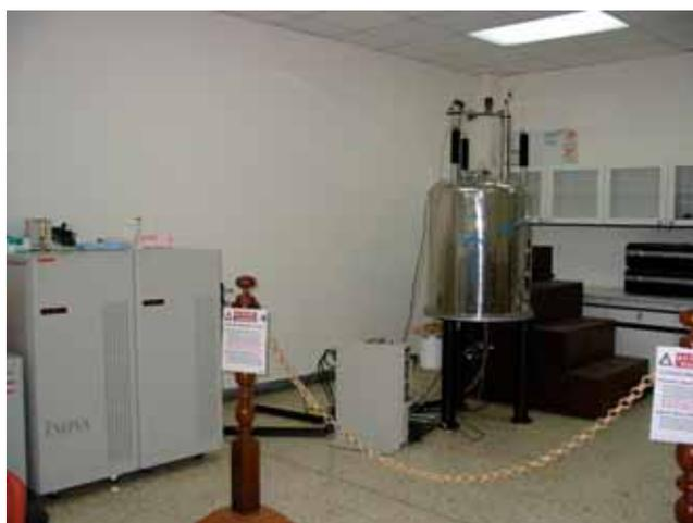
**Figure 3.5** 300 MHz Unity Inova NMR spectrometer.
