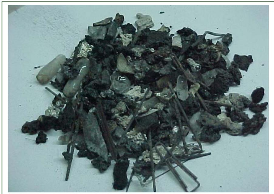
**Figure 4.3.** Bottom ash components with particle size of 4.75-9.5 mm
