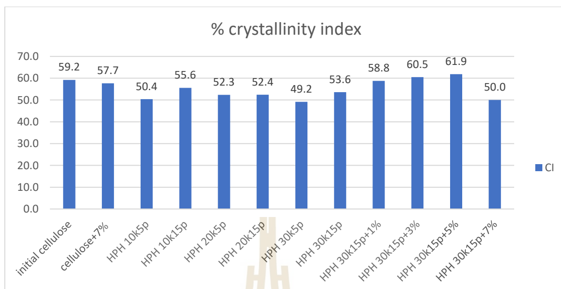
Figure 4.10 crystallinity index of cellulose in different methods.
