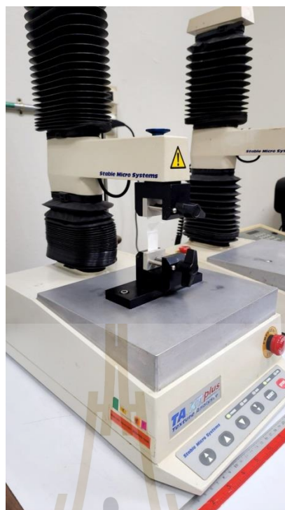
Figure 3.9 A TA.XT Plus SMS Stable Micro Systems Texture Analyzer (Stable Microsystems Ltd., Surrey, England)
