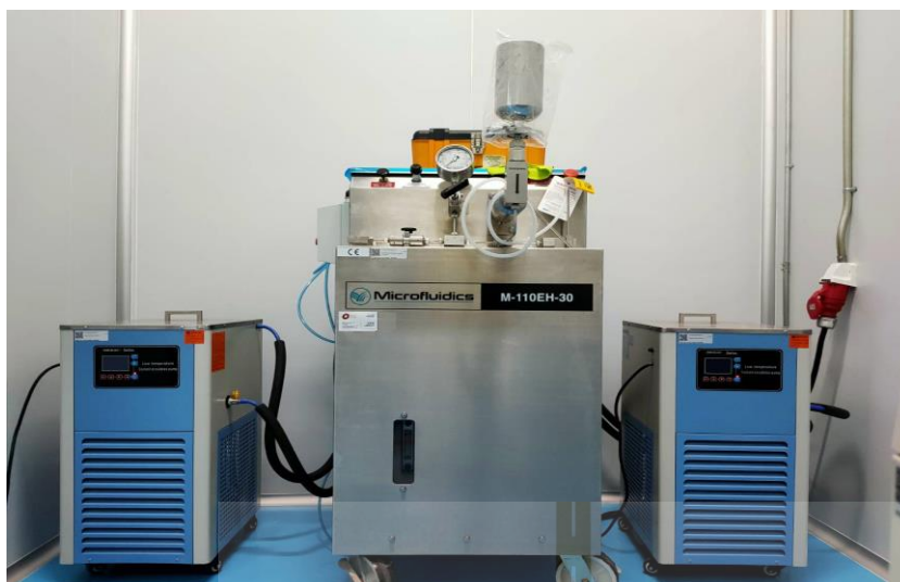
Figure 3.1 Hydraulic pilot-scale homogenizer (Microfluidics, M-110EH-30, USA)
