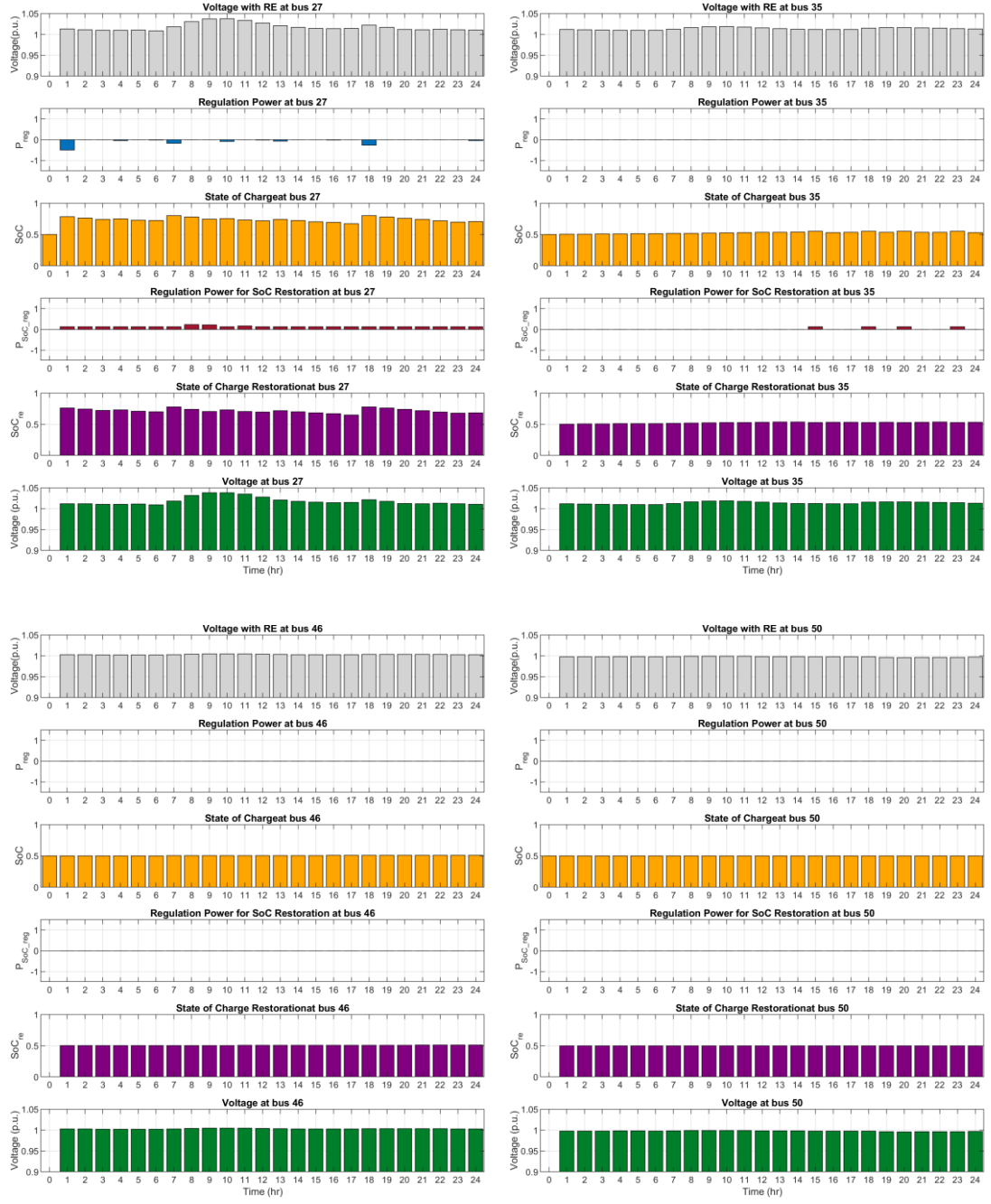
Figure A.9 Time-Series Profiles of Voltage, Regulation Power and Battery SoC at Bus 27, 35, 46 and 50 in IEEE 69-bus system Scenario 2
