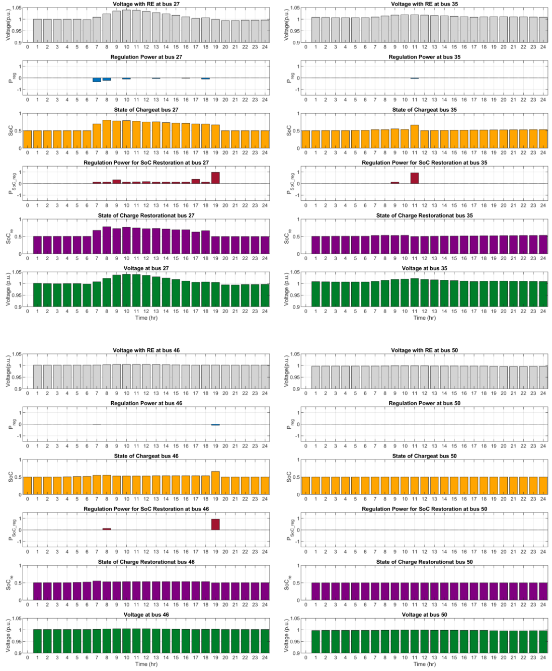
Figure A.11 Time-Series Profiles of Voltage, Regulation Power and Battery SoC at Bus 27, 35, 46 and 50 in IEEE 69-bus system Scenario 3
