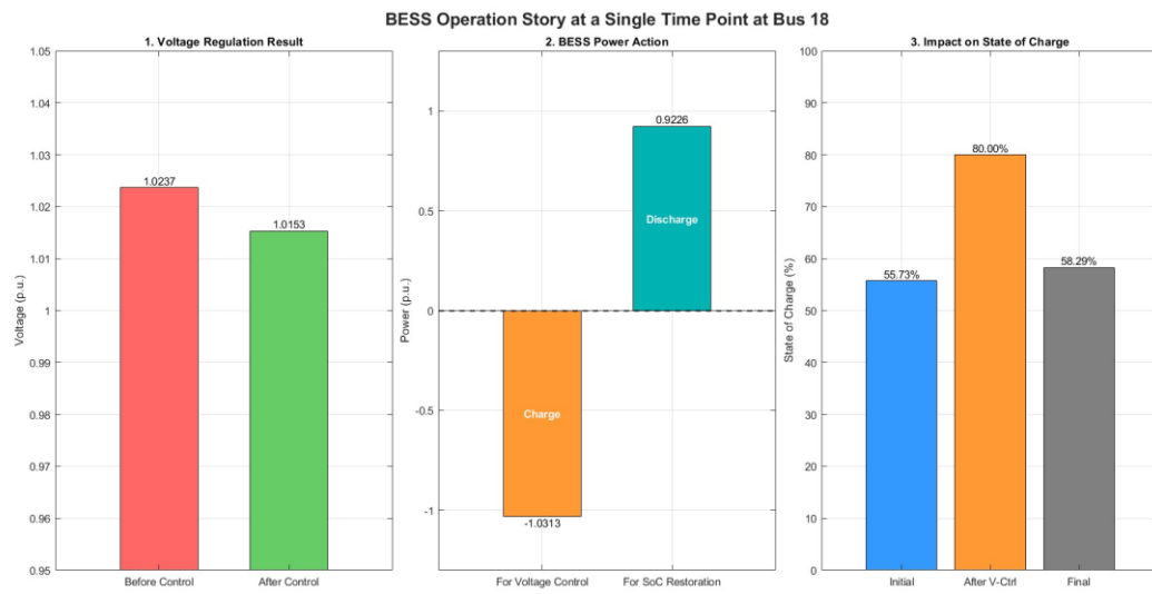
Figure 5.17 Overview of BESS Operation for Voltage Support scenario 3
