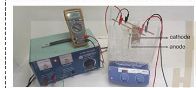
Figure 2 Electrolytic polishing experimental setup.
