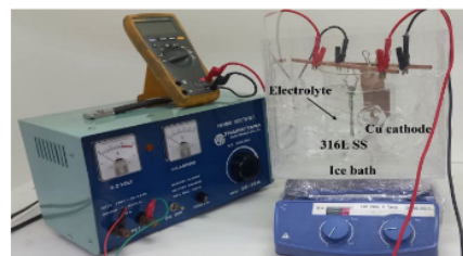
Figure 2. Electrolytic polishing experimental setup with a cooling bath.
