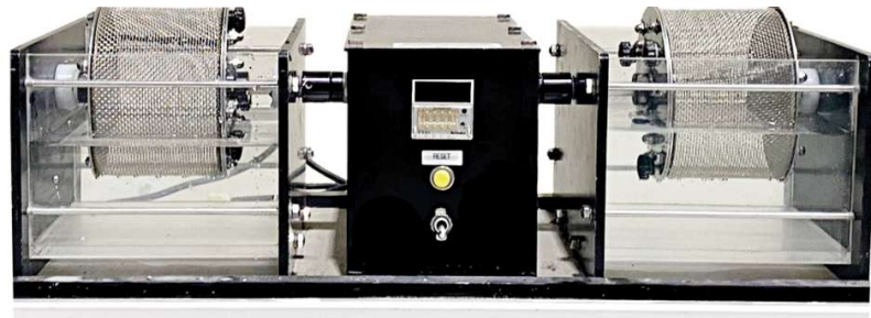
Figure 4.2 Slake durability index test apparatus.
