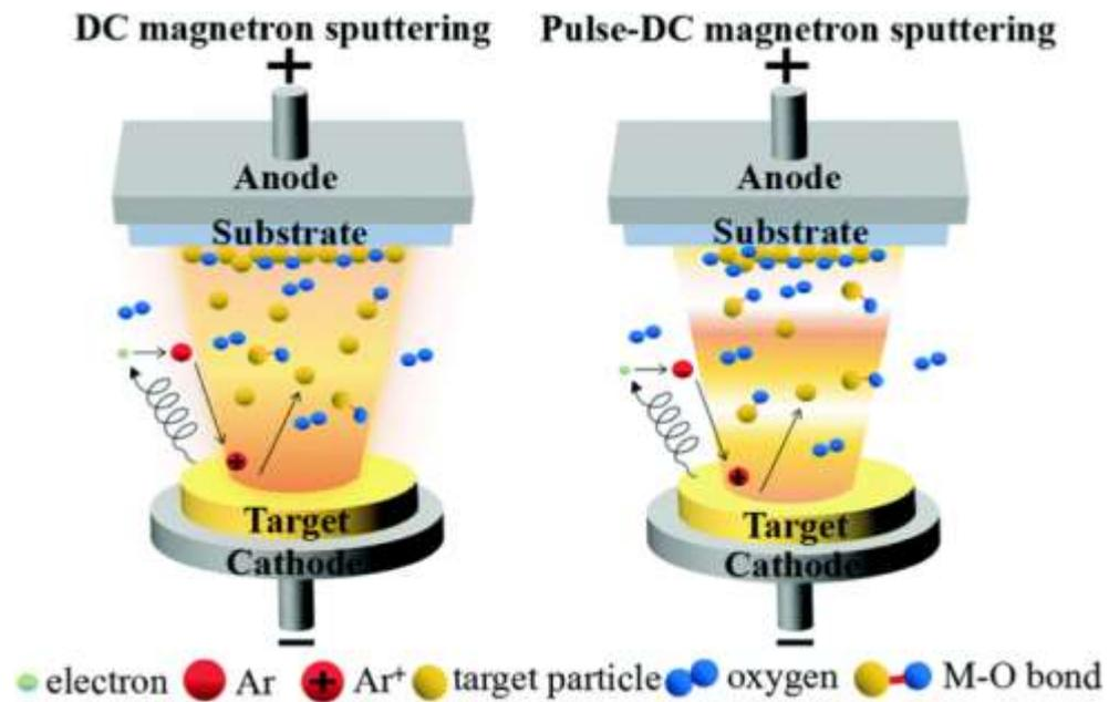
Figure 11 DC magnetron sputtering and. Pulsed DC magnetron sputtering (Vaccoat, 2024).
