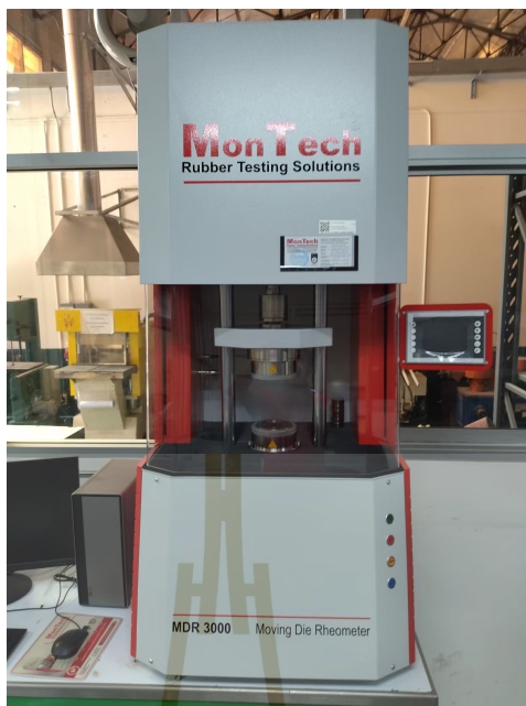
Figure 3.4 MDR 3000 moving die rheometer is used to determine curing time of composite material.
