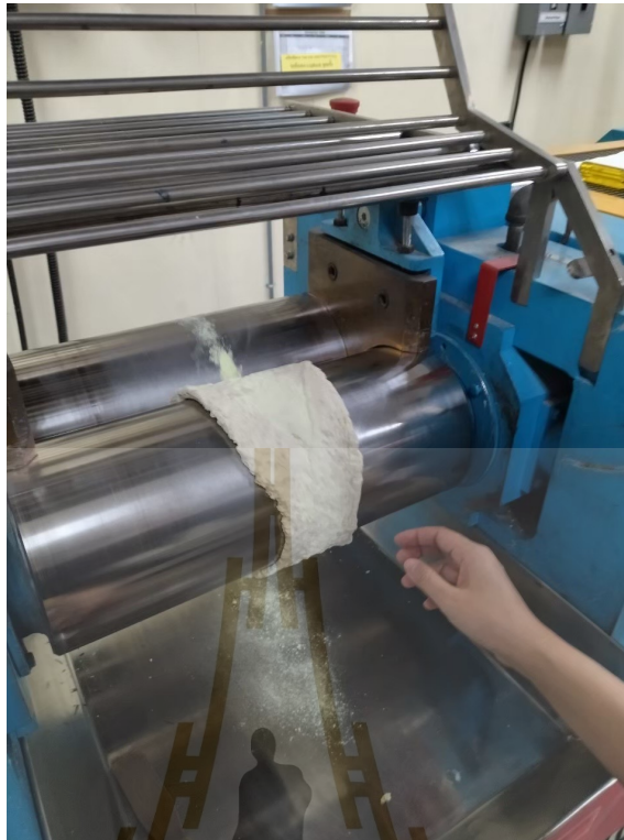
Figure 3.3 Two roll mill is the equipment for mix sulfur into composite materials and shape samples into sheets.
