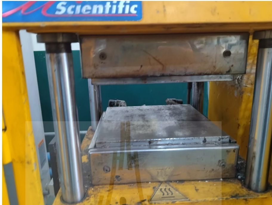
Figure 3.6 A compression molding machine model LP20-B from Labtech Engineering Company Ltd. was used for vulcanizing the sample.
