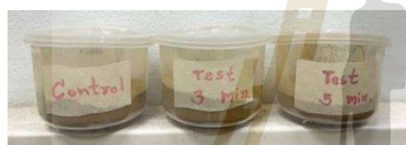
Fig. 2. Lead contaminated soils under test.
