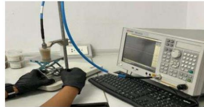
Fig. 3. Measuring of the dielectric properties of a soil under test with a dielectric meter.
