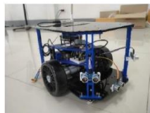
Figure 1. Real robot model (Lapras robot) with all sensors, devices and parts.
