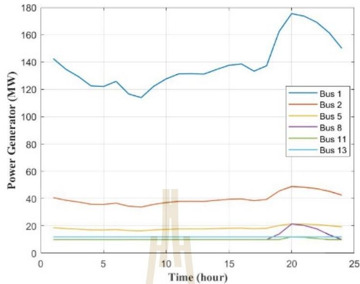
Figure. 4.8 Hourly power generator for case IV
