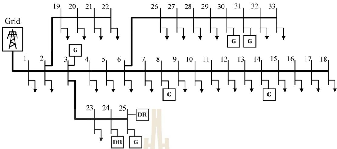
Figure 3.1 The modified IEEE 33-Bus system
