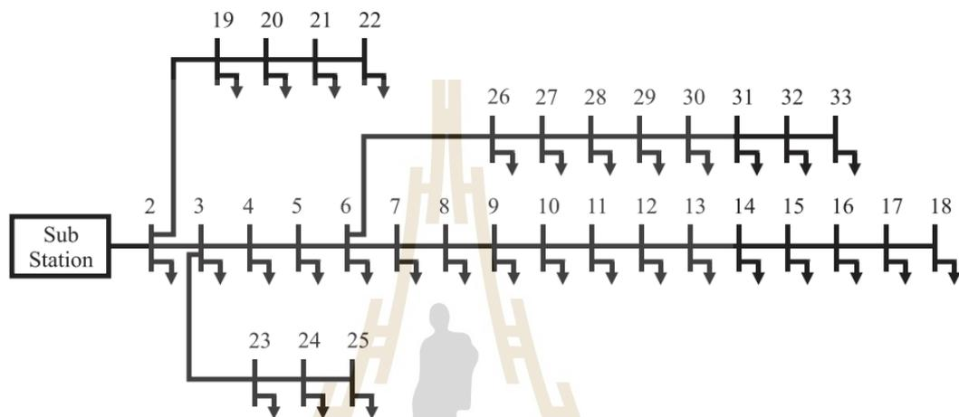
Figure A.1 The IEEE 33 bus system network diagram.
