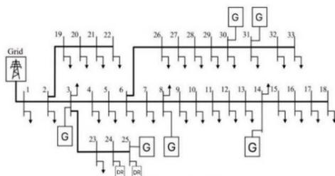
Fig. 1. The modified IEEE 33-Bus system
