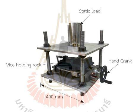
Figure 4.1 Test apparatus used in this study based on West apparatus (West, 1989).
