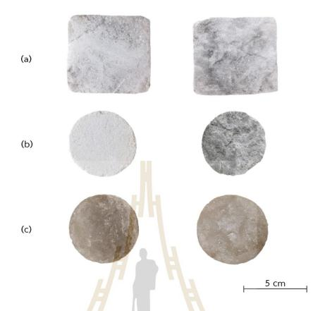
Figure 3.4 Rock samples used in CERCHAR test on smooth (left side) and rough (right side) surfaces in sulfate and chloride group, Suratthani gypsum (a), Nakhon Si Thammarat gypsum (b), and rock salt (c).
