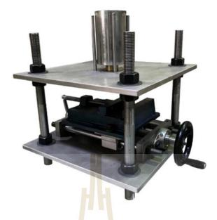
Figure 1.2 Test apparatus used in this study based on West apparatus (West, 1989).
