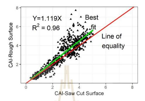
Figure 2.4 Correlation between CAI-Rough surface and CAI-Saw cut surface (Aydın, 2019).
