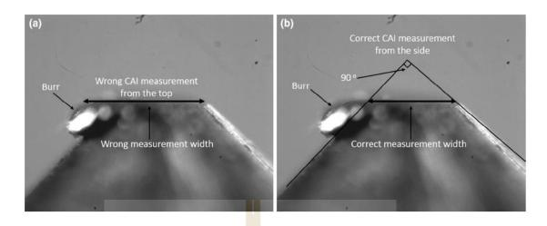
Figure 2.5 View of pin tip wear surface measured from the top view (a) and the side view (b) (Rostami et al., 2014).
