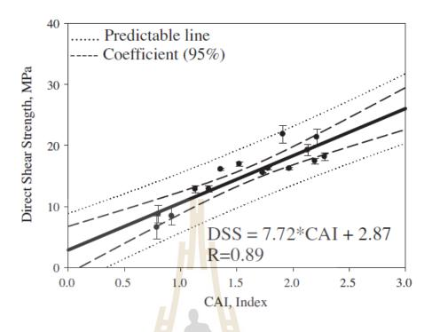
Figure 2.8 Relationship between CAI and direct shear strength (Deliormanlı, 2012).
