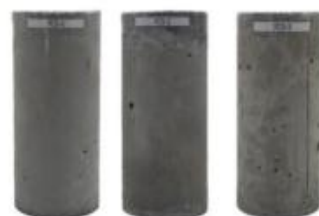
(a) Grouting cement samples
