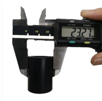
Figure 3.7 Heater bypass cap for plugging grouting material.
