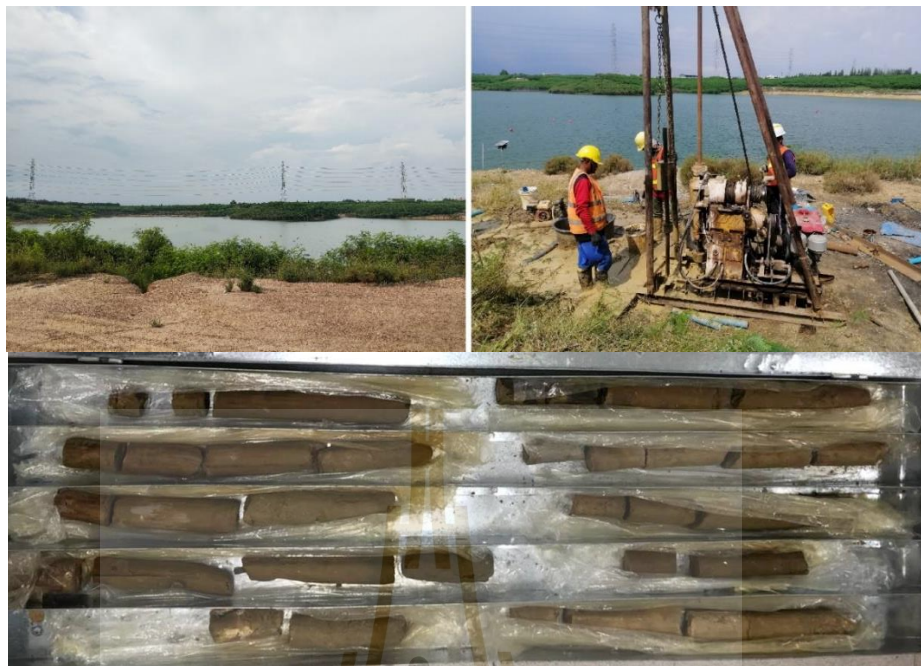
Figure 3.6 The drilling site of Borehole KU4 and examples of sediments, range from 5.0 – 10.0 meters depth (photo by Chatchalerm Ketwetsuriya)
