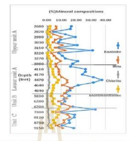
Figure 4. Clay mineral composition of FA-SS-35-04 well with depth.
