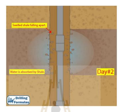
Figure 2.7 Day 2 # Shale swelling due to water and shale starts falling apart. (DrillingFormulas.Com, 2011).
