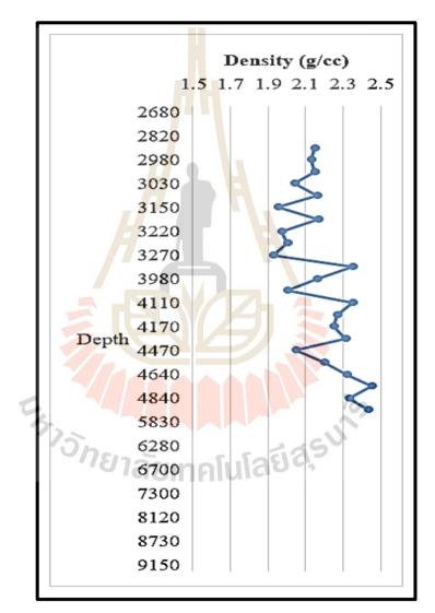
Figure 4.6 Density data from FA-SS-35-04 well from Density log.
