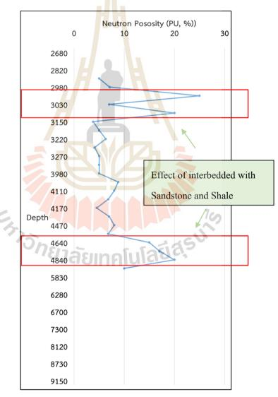
Figure 4.7 The volume from the neutron log of FA-SS-35-04 well from the Neutron log.
