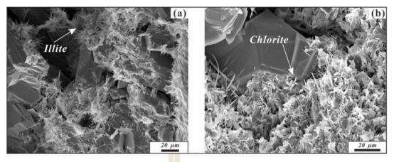
Figure 2.12 SEM image of illite (a) and chlorite (b) (Kun Yu, et al., 2019).
