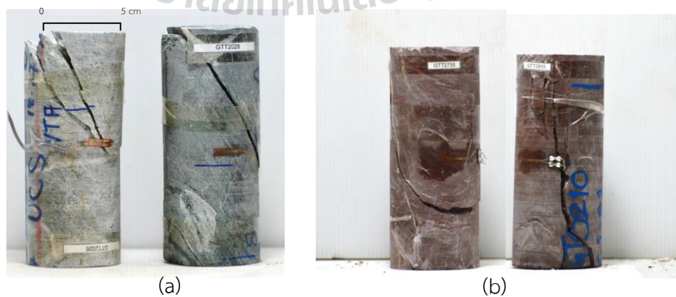
Figure 3.7 Post-test VTF (a) and SLR (b) specimens of UCS testing.
