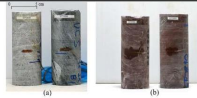
Fig.3. Some VTF (a) and SLR (b) specimens prepared for UCS testing.
