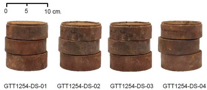
Figure 3.19 Soil samples after testing
