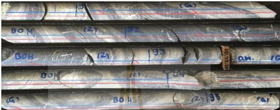
Figure 2.7 Typical SLS cores with characteristic foliation, local folding and carbonate.
