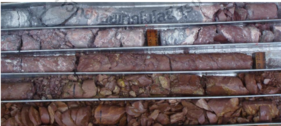
Figure 2.17 Black Fault 16 with black, clayey matrix supported fault breccia in VTF.
