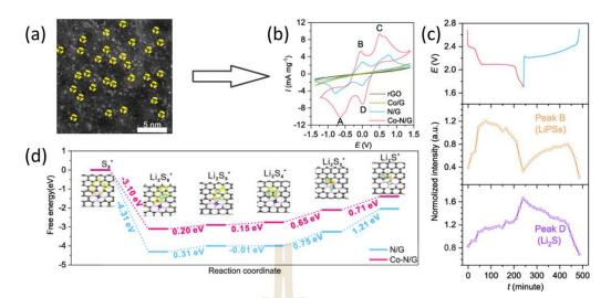
**Figure 1.6** (a) HAADF-STEM image of Co-N doped graphene. (b) CV of symmetric cell with Co and N doping, N doping, and Co doping on graphene for Li-S battery. (c) Evolution of the intensities of peak B and peak D. (d) Energy profiles for LiPS on N-doped and Co-N-doped graphene (Z. Du *et al.*, 2019).
