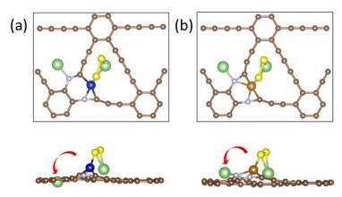
**Figure 5.4** Top and side views for dissociation of Li-S bond of  $Li_2S_2$  on (a)  $CoN_2@GDY$  and (b)  $FeN_2@GDY$ . These configurations are the same as site B in Figure 5.3c. Brown, C; light blue, N; yellow, S; green, Li; blue, Co; gold, Fe.
