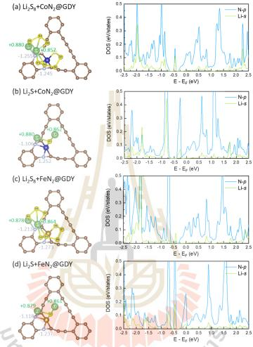
**Figure 4.5** Bader charge distribution upon adsorption (left panel) and corresponding partial density of state (right panel) of Li and N for (a)  $Li_2S_8$  and (b)  $Li_2S$  adsorbed  $CoN_2@GDY$ , and (c)  $Li_2S_8$  and (d)  $Li_2S$  adsorbed  $FeN_2@GDY$ .
