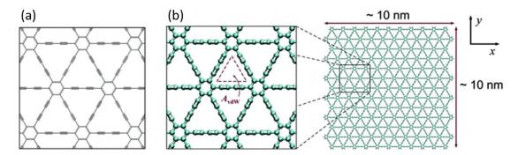
**Figure 1.3** (a) chemical Lewis's structure of graphduyne (GDY). (b) Full atomistic model of GDY depicting the triangular **po**re (Cranford *et al.*, 2012).
