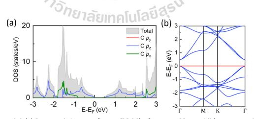
**Figure 3.2** (a) Projected density of state (PDOS) of pristine GDY and (b) corresponding electronic band structure.
