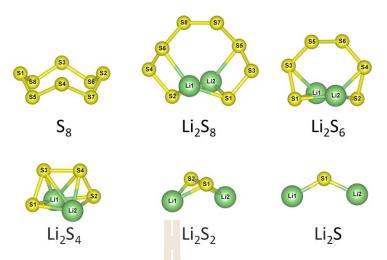
Figure 4.1 The relaxed molecular structures of  $S_8$  and LiPS species. Li and S atoms are represented by green and yellow spheres, respectively.
