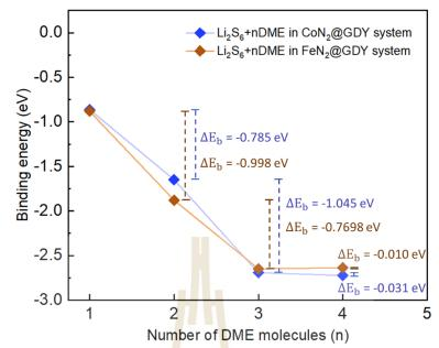
**Figure 4.8** The difference of binding energies between Li2S6 and DME molecule(s) in the co-adsorption systems of CoN2@GDY (blue line) and FeN2@GDY (brown line).
