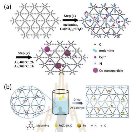
**Figure 1.7** Schematic illustration of the synthetic procedure of (a) Co-N doped GDY (X. Wang *et al.*, 2019) and (b) Fe-N doped GDY (Si *et al.*, 2019) from experimental views.
