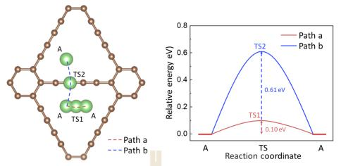
**Figure 5.6** Diffusion of Li-ion along path a (red dash line) and path b (blue dash line), left panel. The corresponding energy profile along the path a (red solid line) and path b (blue solid line), right panel. Color code: brown, C; green, Li.
