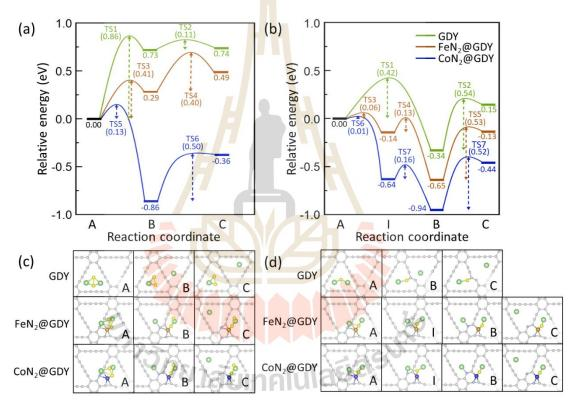
**Figure 5.3** Potential energy profiles of (a)  $Li_2S_2$  and (b)  $Li_2S$  decompositions on GDY (green line),  $CoN_2@GDY$  (blue line), and  $FeN_2@GDY$  (yellow line), and their corresponding intermediates for (c)  $Li_2S_2$  and (d)  $Li_2S$  decompositions. The labeled numbers at the intermediate states indicate their relative energies, whereas the numbers in parentheses denote the energy barriers.
