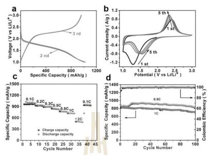
**Figure 1.5** (a) The 2<sup>nd</sup> and 3ed charge/discharge of SGDY cathode at 0.1 C (1 C = 1672 mA g<sup>-1</sup>). (b) CV curve at a scan rate of 0.1 mV s<sup>-1</sup>. (c) Rate performance. (d) Cycling performance of SGDY cathode at current densities of 0.5 and 1 C (H. Du *et al.*, 2017).
