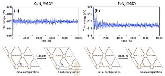
Figure 3.4 The variation of total energy as a function of time along AIMD simulation at 300 K and corresponding initial and final configurations of (a)  $CoN_2@GDY$  and (b)  $FeN_2@GDY$ .
