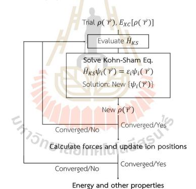
Figure 2.2 The scheme of self-consistency iteration for solving the Kohn-Sham equation and obtaining the calculated total energy and other properties (Modified
