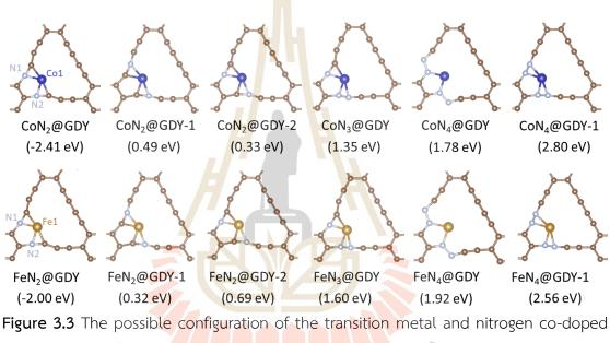
GDY. Note that the corresponding formation energy of each configuration is shown in parentheses. C, N, Co, and Fe atoms are represented by brown, grey, blue, and gold, respectively.
