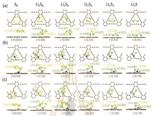
**Figure 4.3** Top and side views of the most stable adsorption configurations of  $S_8$  and LiPSs on (a) pristine GDY, (b)  $CoN_2@GDY$ , (c)  $FeN_2@GDY$ . Brown, C; light blue, N; yellow, S; green, Li; blue, Co; gold, Fe. Charges of each Li atom, all S atoms, and the substrate are labelled in green, yellow, and brown numbers, respectively.
