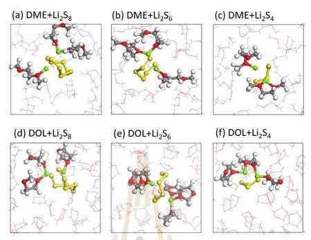
**Figure 5.1** Low-energy configurations of a-c) DME- and d-f) DOL-solvated LiPSs as obtained from AIMD simulations. Illustrations in the ball-and-stick model represent electrolyte molecules in the first solvation shell, whereas the wireframe models are the outer solvation shell.
