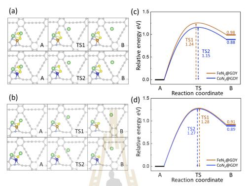
**Figure 5.5** Another reaction path of catalytic decomposition of (a)  $Li_2S_2$  and (b)  $Li_2S$ , and corresponding energy profile of (c)  $Li_2S_2$  and (d)  $Li_2S$ , respectively, on  $CoN_2@GDY$  (blue line) and  $FeN_2@GDY$  (yellow line). Color code: gray, C; light blue, N; yellow, S; green, Li; blue, Co; gold, Fe.
