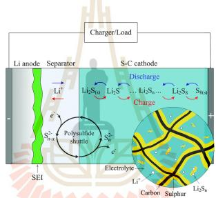
**Figure 1.2** Summary of the effect on electrodes, including the lithium polysulfide shuttle, polysulfide dissolution, and insoluble phase SEI formation on the anode side (Wild *et al.*, 2015).
