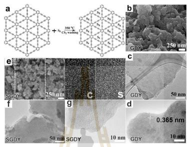
**Figure 1.4** (a) The schematic of the preparation process of sulfide graphdiyne (SGDY). (b) SEM image of GDY. (c) TEM image of GDY. (d) HRTEM image of GDY. (e) SEM image of SGDY. (f) TEM image of SGDY. (g) HRTEM image of SGDY (H. Du *et al.,* 2017).
