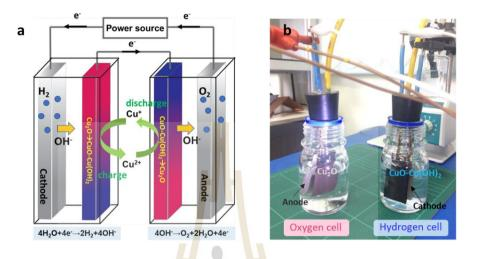
**Figure 3.6** The membrane-free configuration for alkaline water electrolysis in separate oxygen and hydrogen cell. (a) Schematic illustration and (b) experimental setup of a two-cell water electrolysis system after operated 20 minutes, respectively.
