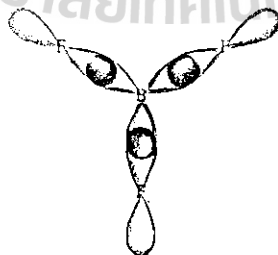
Figure 12 Overlap of the sp^2 hybrid orbitals of the boron atom with the 2p orbitals of the fluorine atoms. The \text{BF}_3 molecule is planar, and all the \text{FBF} angles are 120^\circ .
