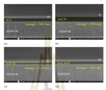
Fig. 3. FIB-SEM images of (a) ta-C, (b) ta-C:N, (c) ta-C:Al, and (d) ta-C:Al:N.
