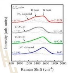
Fig. 2. Reman spectra of ta-C, ta-C:N, ta-C:Al, and ta-C:Al-N.
