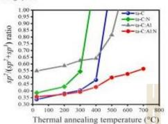
Fig. 11. ta-C, ta-C:N, ta-C:Al, and ta-C:Al:N sp2-hybridized bond fractions plotted as functions of thermal annesling tempe (RT) to graphitization temperature. sature from room term
