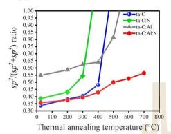
Fig. 11. ta-C, ta-C:N, ta-C:Al, and ta-C:Al:N sp2-hybridized bond fractions plotted as functions of thermal annealing temperature from room temperat (RT) to graphitization temperature.
