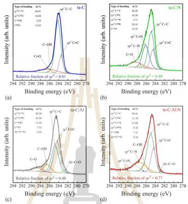
Fig. 6. C 1s XPS spectra and corresponding deconvoluted Gaussian peaks of (a) ta-C; (b) ta-C; N, (c) ta-C; Al, and (d) ta-C; Al:N.
