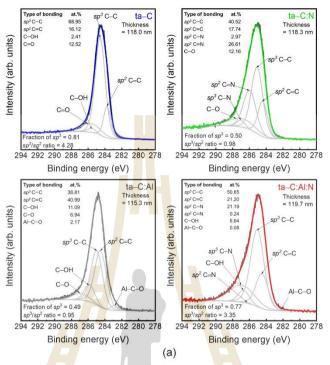
Fig. 5. XPS profiles and deconvoluted Gaussian peaks of the films before the corrosion tests: (a) C 1s, (b) O 1s, (c) N 1s, and (d) Al 2p.
