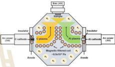
Fig. 1. FCVA deposition system used for the films.
