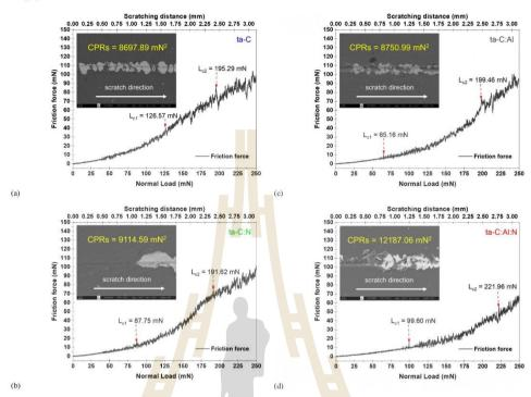
Fig. 11. Scratch curves and SEM images of the scratch tracks at  $L_{c1}$  and  $L_{c2}$  for the films.
