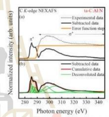
Fig. 9. In-situ high-temperature NEXAES C.K.-edge spectrum generated for ta-C: AEM (a) price to data subtraction (where error function step was applied to fit edge jumping at ionization potential, as indicated in orange) and (b) after data subtraction (where spectrum was deconvoluted into multiple Gaussian peaks).
