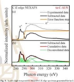
Fig. 9. In-situ high-temperature NEADES C K-edge spectrum generated for ta-C.
