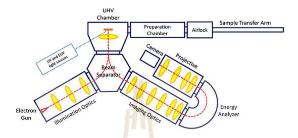
Figure 2.10 The schematic of spectroscopic photoemission and low electron microscope (SPELEEM) [Online], Available: https://groups.oist.jp/fsu/leem-peem
