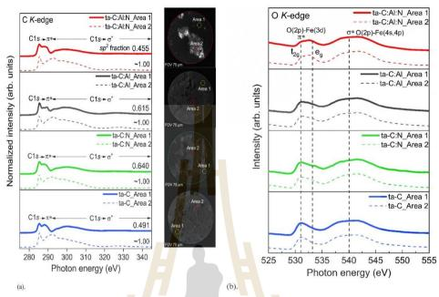
Fig. 10. NEXAFS spectra of the films after the corrosion tests: (a) C K-edge, (b) O K-edge, (c) N K-edge, and (d) Fe L<sub>3,2</sub>-edge.
