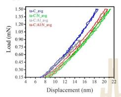
Fig. 5. Load-displacement curves of ta-C, ta-C:N, ta-C:Al, and ta-C:Al:N.
