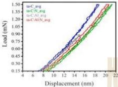
Fig. 5. Load-displacement curves of ta-C, ta-CN, ta-CAI, and ta-CAI:N.
