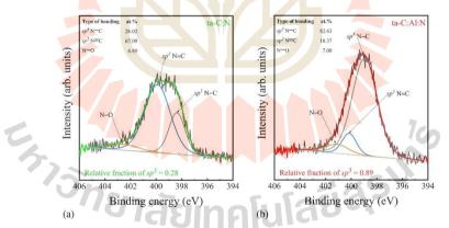
Fig. 7. N 1s XPS spectra and corresponding deconvoluted Gaussian peaks of (a) ta-C:N and (b) ta-C:Al:N.
