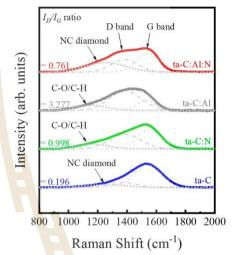
Fig. 2. Raman spectra of ta-C, ta-C:N, ta-C:Al, and ta-C:Al:N.
