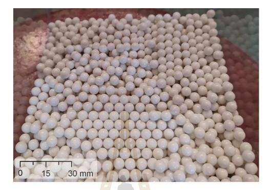
Figure 3.1 ABS balls with uniform sizes of 6 mm used to simulate cavern roof and
