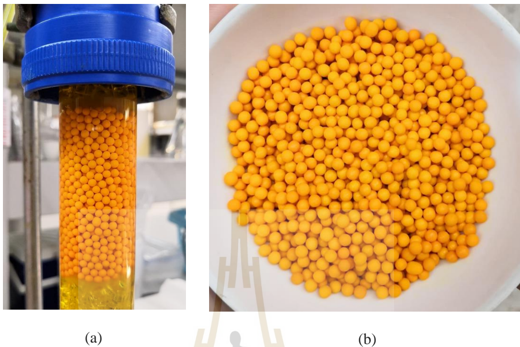
Figure 5.14 Synthetic clay adsorbent in non-aqueous adsorption of methyl orange: (a) in the fixed-bed column, (b) after adsorption.
