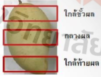
Figure 3 Position of firmness test
