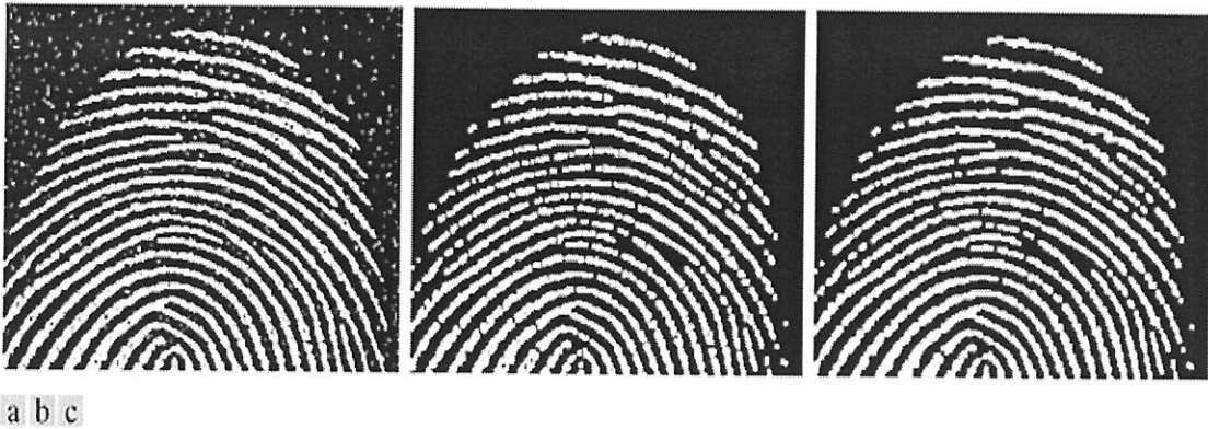
FIGURE 9.11 (a) Noisy fingerprint image. (b) Opening of image. (c) Opening followed by closing. (Original image courtesy of the National Institute of Standards and Technology.)
