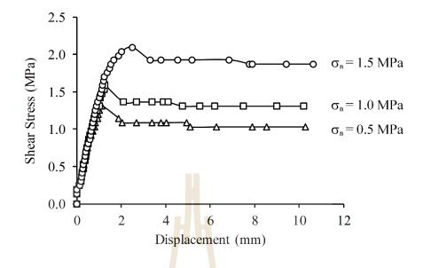
**Figure 5.16** Shear stress as a function of shear displacement for RHA:C = 10:10.
