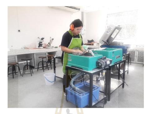
Figure 5.1 Cylindrical specimens are prepared to the desired length with L/D ratio between 2.0 to 2.5.
