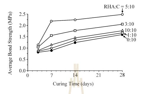
Figure 5.20 Average bond strength as a function of curing time.
