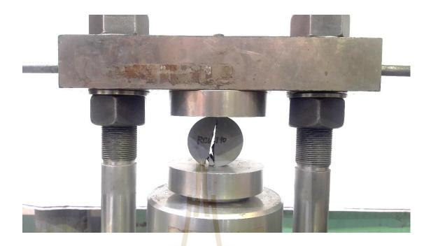
Figure 5.7 Brazilian tensile strength test with constant loading rate.
