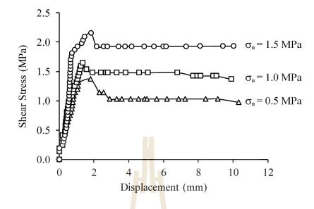
**Figure 5.14** Shear stress as a function of shear displacement for RHA:C = 3:10.
