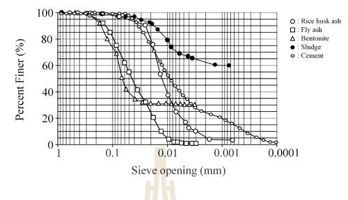
Figure 3.2 The particle size distribution of rice husk ash compared with those of fly
