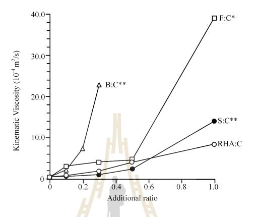
Figure 4.7 Kinematic viscosity of mixture material for different ratios (\*Chiangmai,
