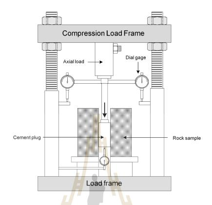
Figure 5.18 Schematic drawing of push-out test.
