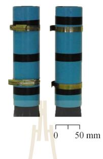
Figure 3.4 PVC molds with curing cement mixture.
