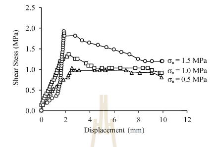
Figure 5.12 Shear stress as a function of shear displacement for pure cement.
