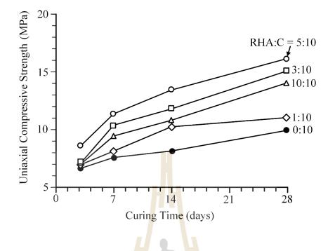
Figure 5.4 Uniaxial compressive strengths of grouting materials as a function of curing
