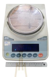
Figure 4.3 Digital weight scale with maximum capacity of 2,200 g and accuracy to
