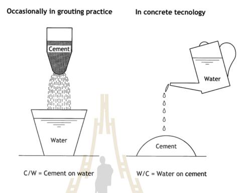
**Figure 2.1** Definition of the water to cement ratio (W/C) (Deere, 1982).
