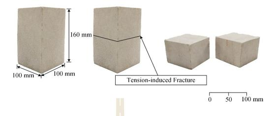
Figure 3.6 Some sandstone samples are prepared for direct shear test.
