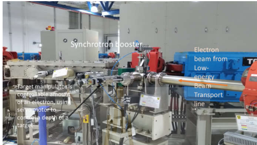
Figure 3.1 Target manipulator for controlling amount of an electron.
