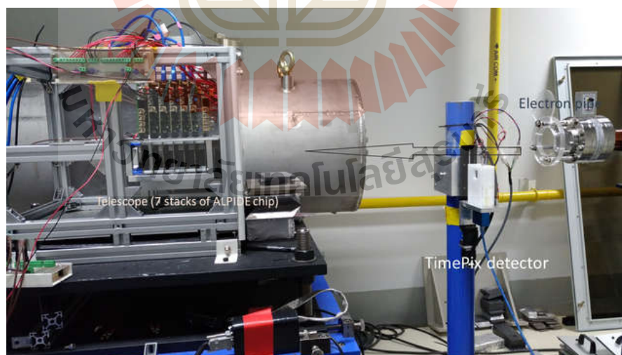
Figure 3.2 Beam Test station layout at Synchrotron Light Research Institute Beam Test Facility.
