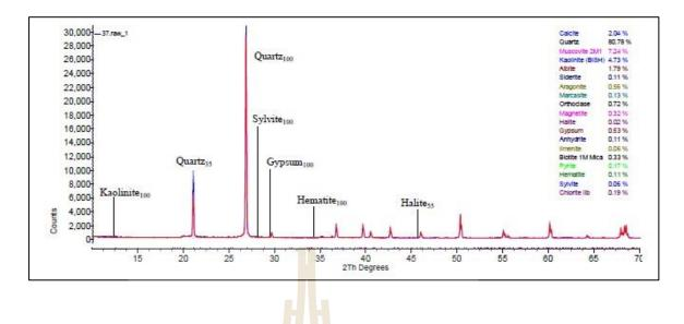
Figure B.31 Interpretation of X-Ray Diffractometer analysis from site number 37.
