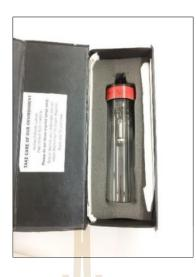
**Figure 3.10** Hollow cathode lamp.
