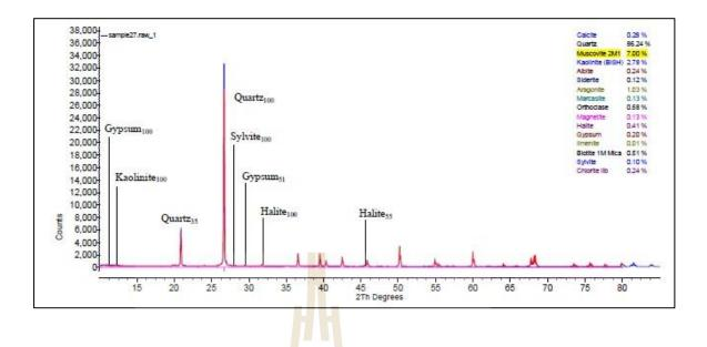
Figure B.23 Interpretation of X-Ray Diffractometer analysis from site number 27.
