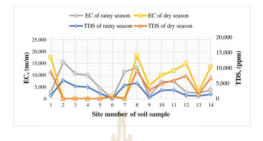
Figure 4.6 The electrical conductivity (EC) and total dissolved solids (TDS) of soil
