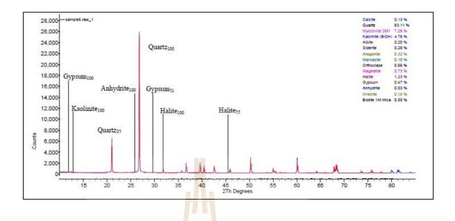
Figure B.3 Interpretation of X-Ray Diffractometer analysis from site number 5.
