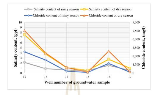
Figure 4.24 The salinity content and chloride content of groundwater samples at Non
