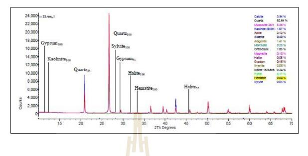
Figure B.29 Interpretation of X-Ray Diffractometer analysis from site number 33.
