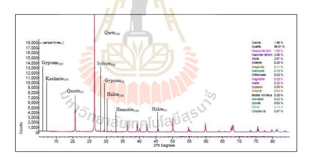
Figure B.16 Interpretation of X-Ray Diffractometer analysis from site number 19.
