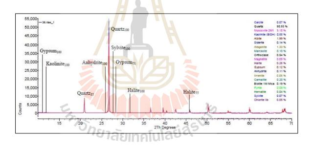
Figure B.30 Interpretation of X-Ray Diffractometer analysis from site number 36.
