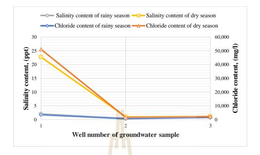
Figure 4.22 The salinity content and chloride content of groundwater samples at Non
