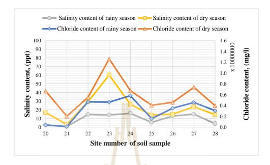
Figure 4.19 The salinity content and chloride content of soil samples at Non Sung
