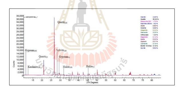
Figure B.24 Interpretation of X-Ray Diffractometer analysis from site number 28.
