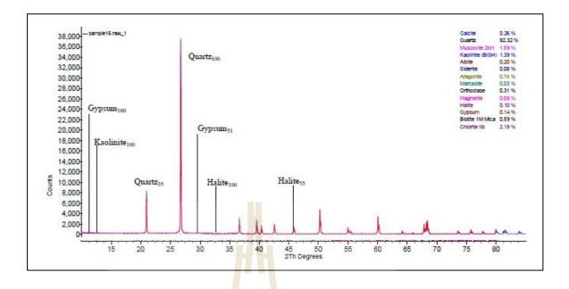
Figure B.13 Interpretation of X-Ray Diffractometer analysis from site number 16.
