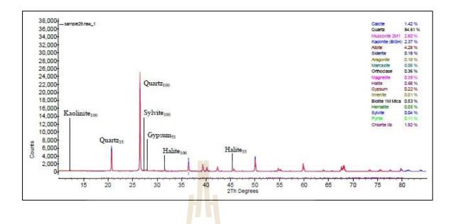
**Figure B.25** Interpretation of X-Ray Diffractometer analysis from site number 29.
