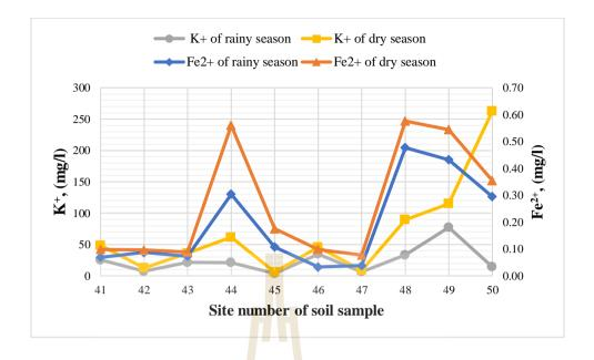
Figure 4.41 Contents of potassium and iron ions of soil samples at Kham Sakae Saeng
