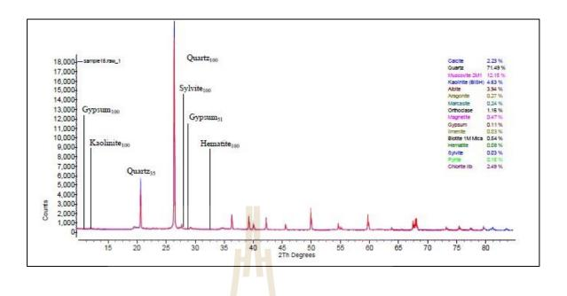
**Figure B.15** Interpretation of X-Ray Diffractometer analysis from site number 18.
