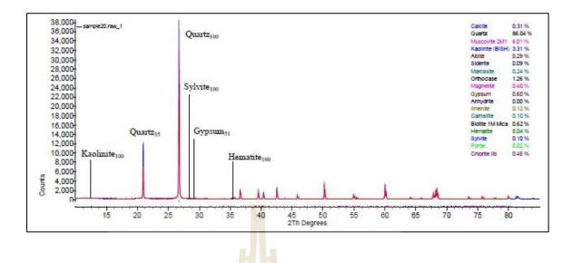
Figure B.17 Interpretation of X-Ray Diffractometer analysis from site number 20.
