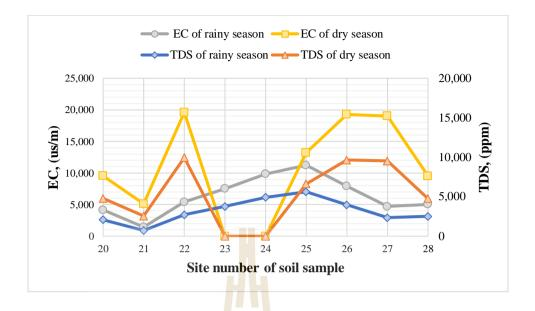
Figure 4.8 The electrical conductivity (EC) and total dissolved solids (TDS) of soil
