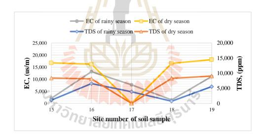
Figure 4.7 The electrical conductivity (EC) and total dissolved solids (TDS) of soil samples at Non Thai district.
