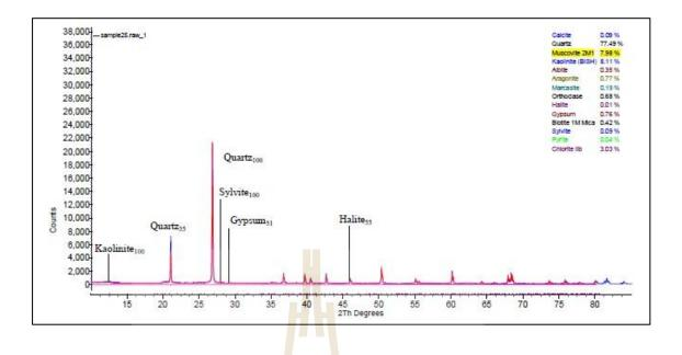
Figure B.21 Interpretation of X-Ray Diffractometer analysis from site number 25.
