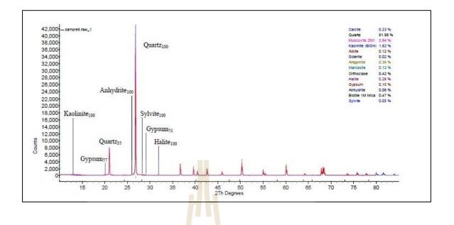
Figure B.5 Interpretation of X-Ray Diffractometer analysis from site number 8.
