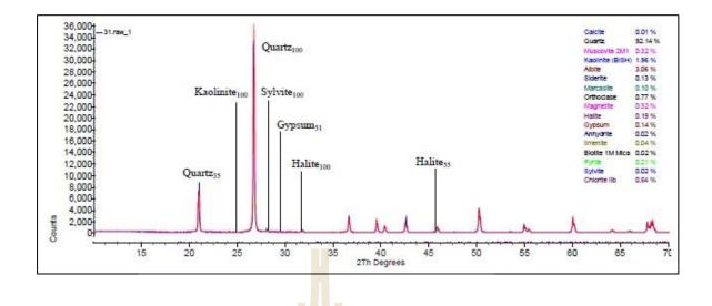
Figure B.27 Interpretation of X-Ray Diffractometer analysis from site number 31.
