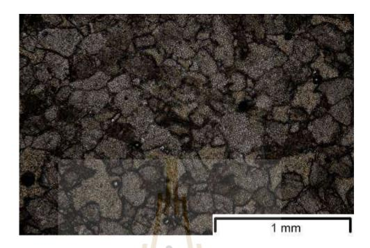
Figure 3.27 PPL-photomicrograph of the white quartz sandstone.
