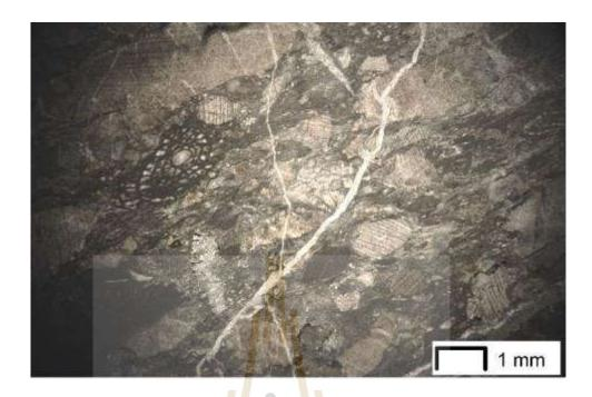
**Figure 3.15** PPL-photomicrograph of the limestone 2.
