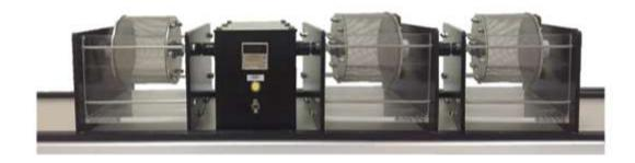
Figure 4.1 Slake durability index test apparatus.
