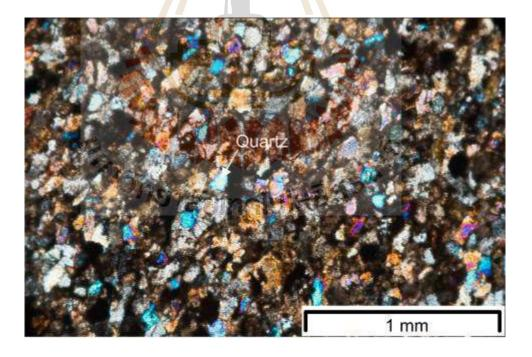
Figure 3.24 XPL-photomicrograph of the quartz sandstone.
