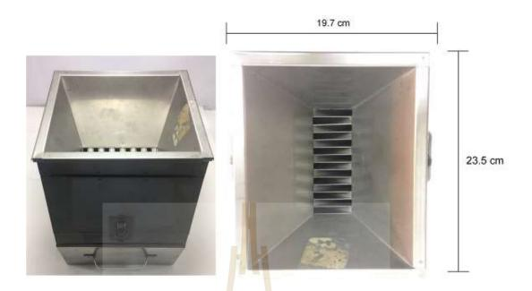
Figure 5.12 Chute splitter for sample separation.
