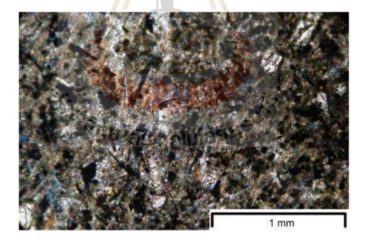
Figure 3.8 XPL-photomicrograph of the aphanitic basalt.
