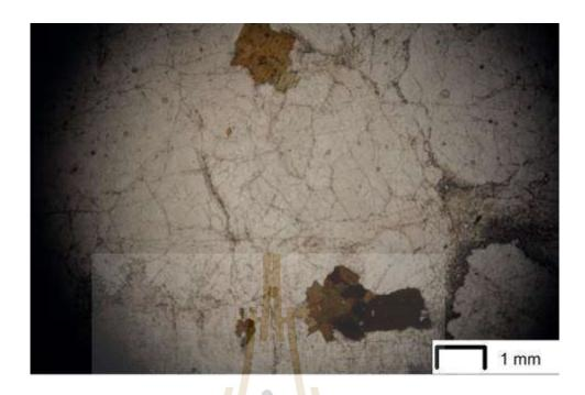
Figure 3.31 PPL-photomicrograph of the white granite.
