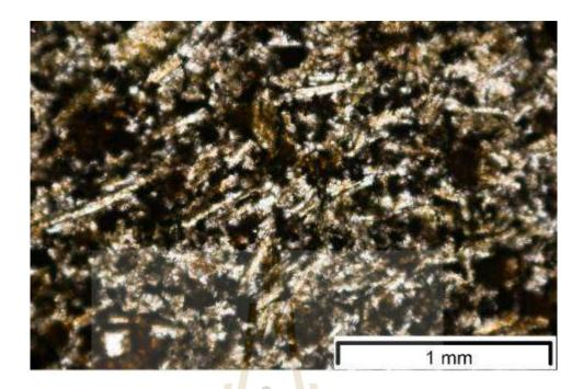
Figure 3.9 PPL-photomicrograph of the ferrous oxide basalt.
