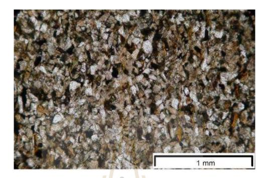
Figure 3.21 PPL-photomicrograph of the calcareous lithic sandstone.
