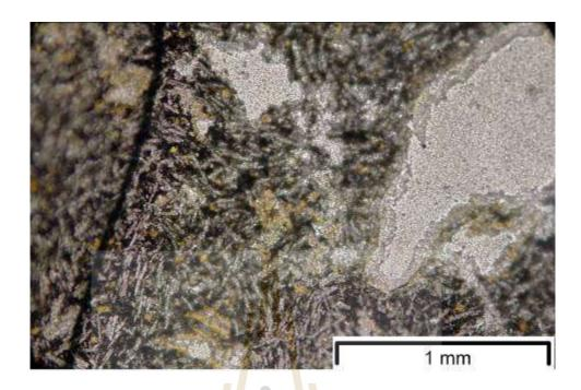
Figure 3.11 PPL-photomicrograph of the vesicular basalt.
