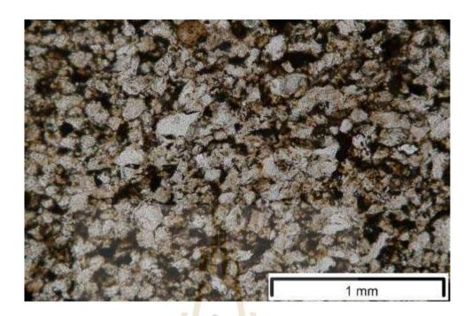
Figure 3.23 PPL-photomicrograph of the quartz sandstone.
