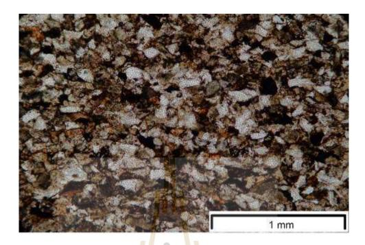
Figure 3.25 PPL-photomicrograph of the arkosic feldspathic sandstone.
