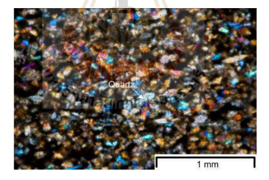
Figure 3.22 XPL-photomicrograph of the calcareous lithic sandstone.
