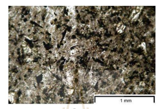
Figure 3.7 PPL-photomicrograph of the aphanitic basalt.
