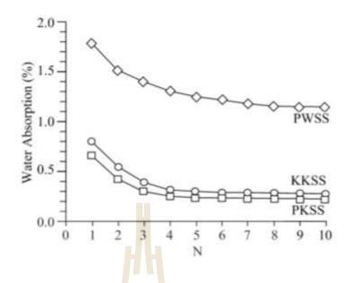
Figure 2.2 Water absorption as a function of test cycles (Walsri et al., 2012).
