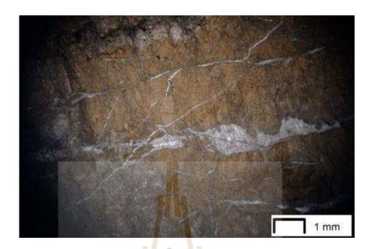
Figure 3.13 PPL-photomicrograph of the limestone 1.
