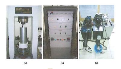
Figure 2.4 TAW-1000 Electro-hydraulic Servo Controlled Testing System: (a) Loading System, (b) Main Switches, (c) Pressure Pumps (Yu et al., 2016)
