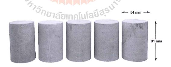
Figure 3.3 Phu Phan sandstone specimens with core axis parallel bedding plane.
