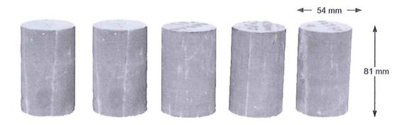
Figure 3.4 Sao Khua sandstone specimens with core axis parallel bedding plane.
