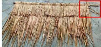
Figure 17 Incomplete sewing at the end of operation.
