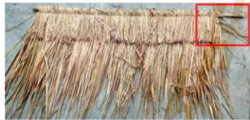
Figure 17. Incomplete sewing at the end of operation
