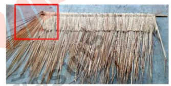
Figure 15. Wrong sewing at the first of operation.
