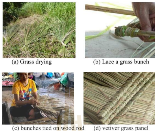
Figure 2. The process of vetiver roofing material manufacturing
