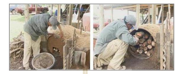
Figure 2.7 Pile Wood in the Kiln (Food and Fertilizer Technology Center, 2005).
