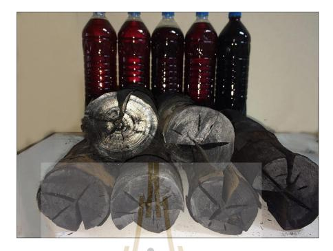
Figure 3.14 Charcoal and wood vinegar obtained from the experiment.
