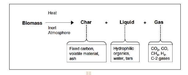
Figure 2.12 A simple representation of pyrolysis process (Iberahim, 2013)
