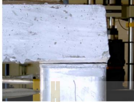
Figure 11 Slab corner tilted upward at failure
