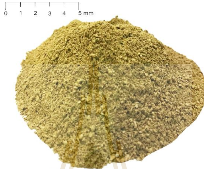
Figure 3.10 Sludge samples from Metropolitan Waterworks Authority.
