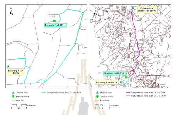
**Figure 4.6** Optimum paths from each TS to DS(s) based on minimization of TC and constraints of 3 (left hand side) and 5 (right hand side) year service life of sites (Continued).
