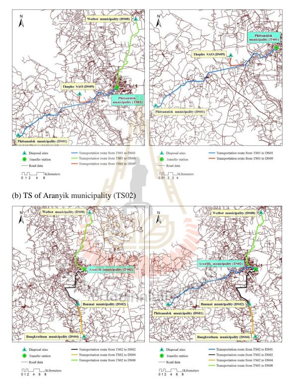
**Figure 4.8** Optimum paths from each TS to DS(s) based on minimization of TC and EI and constraints of 3 (left hand side) and 5 (right hand side) year service life of sites.
