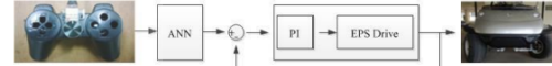
Fig. 3: The operation of human-learning steering control by using artificial neural network (ANN) with steering devices.
