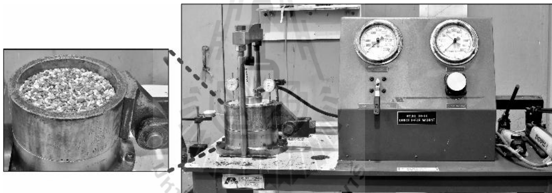
Figure 3.4 Direct shear device SBEL DR44 used in this study.
