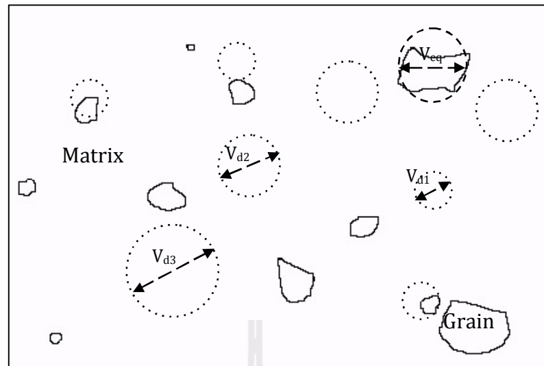
Figure 3.11 Illustration of measurement of grain and void size distributions
