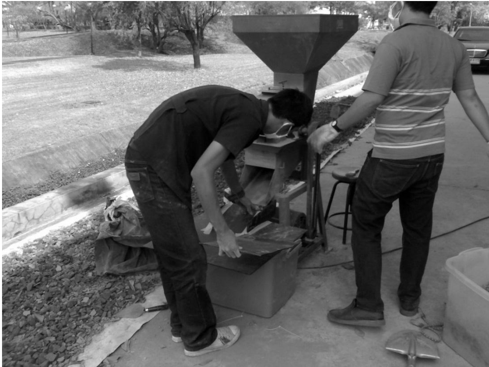
Figure 3.4 Sludge cakes are cracked by a milling machine.
