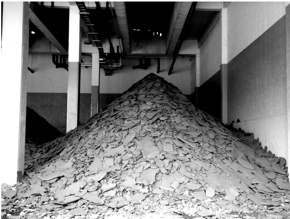
Figure 3.1 Sludge from sludge dewatering plant of Bang Khen Water Treatment Plant located in Bangkok Metropolis.
