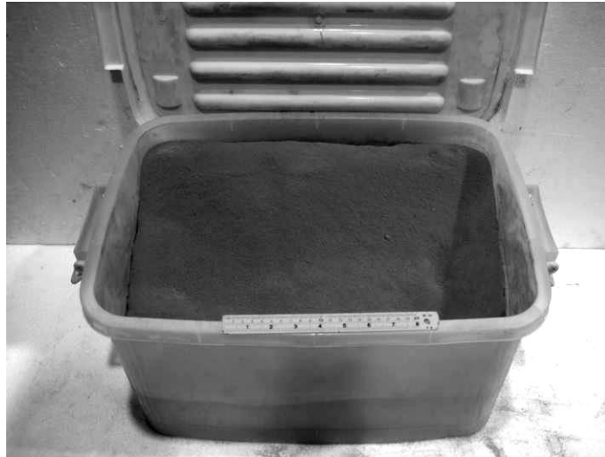
Figure 4.1 Sludge sample packed in a plastic box with a lid to prevent moisture.
