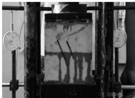
Figure 7. Laboratory arrangement for permeability testing of fractures.
