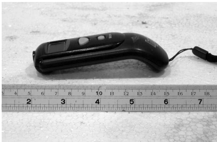
Figure 4.7 Digital thermometer HIP C0905019480 with accuracy to \pm 0.1^{\circ}\text{C} .
