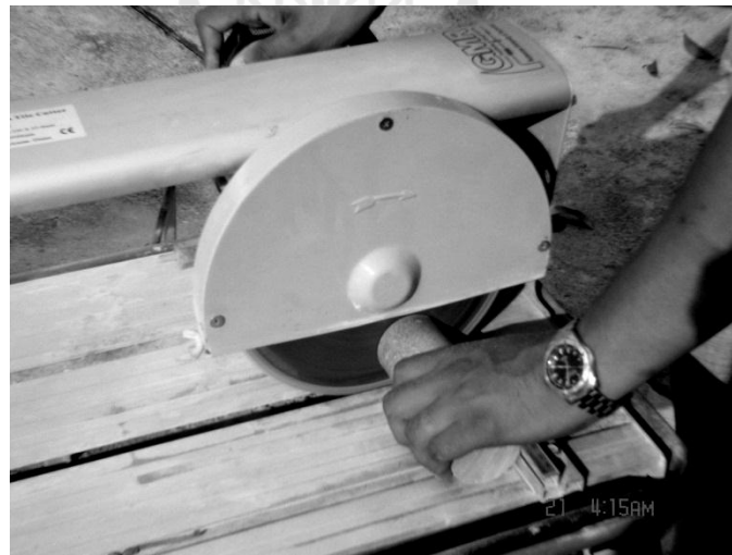
Figure 5.2 Core sample is cut to obtain the desired length with ZE-LG3-570A Tile Cutter.
