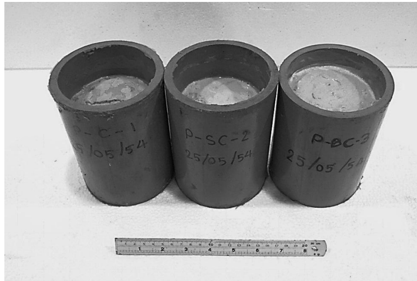
Figure 6.1 PVC mold has an inner diameter of 101.6 mm for permeability testing of grouting materials.
