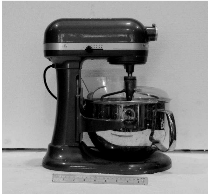
Figure 4.5 Mixer, Kitchenaid Professional 600 6QT 575 watt stand mixer, with maximum capacity for 5,000 cm 3 and 6 speed control.
