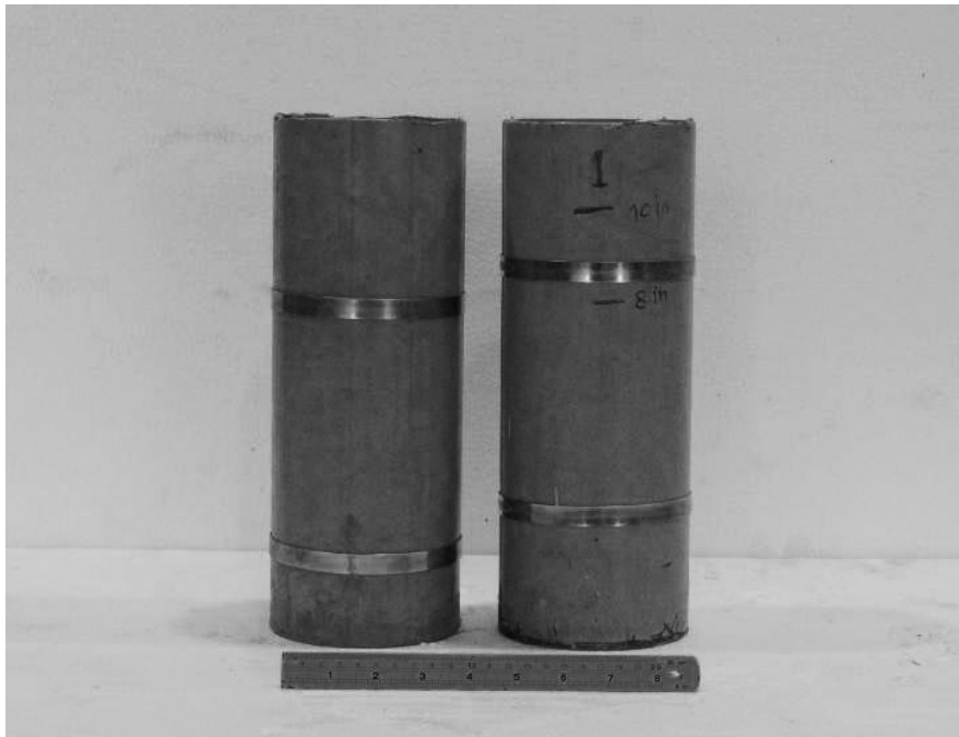
Figure 5.6 PVC mold has an inner diameter of 101.6 mm with 203.2 mm in length.
