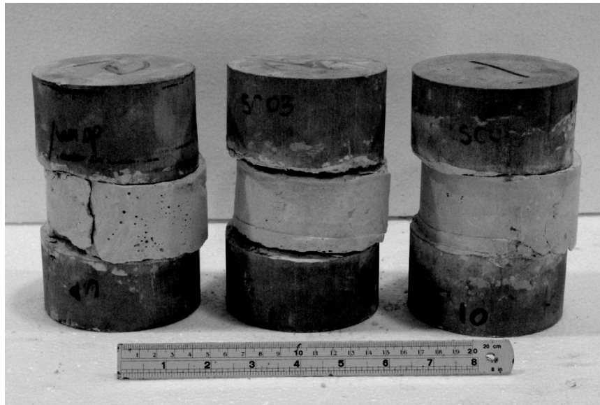
Figure 5.16 Some specimens of grouting material in sandstone fracture after failure under shearing between grout and fracture.
