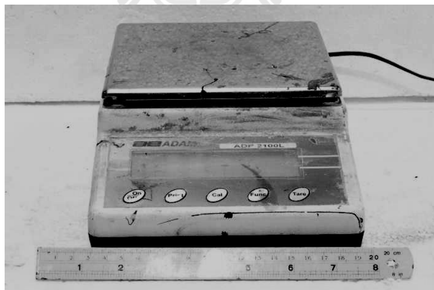
Figure 4.4 Digital weight scale with maximum capacity for 2000 grams and accuracy to \pm 0.01 gram.
