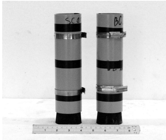
Figure 5.1 PVC mold has an inner diameter of 50.8 mm with a rubber stopper on the bottom.
