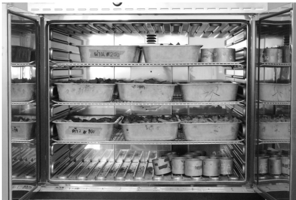
Figure 3.5 Sludge in a hot-air oven at 140°C for at least 24 hours or until its weight remains constant.
