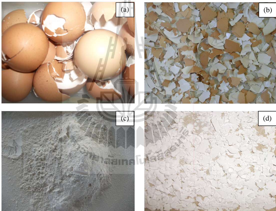
Figure 3.1 Images of ES after cleaning and drying (a), broken ES for preparing ESP and HT-ES (b), ESP (c), and HT-ES (d).
