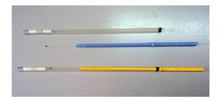
Figure 6. The cryotop vitrification device (Kitazato Supply Co., Tokyo, Japan)
