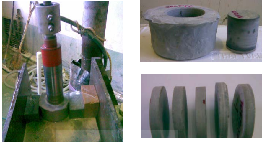
Figure 3.4 Paste specimens coring and cutting for chloride test
