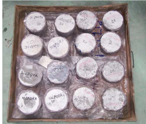
(a) Specimen pastes coated with epoxy
