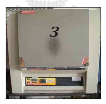
Figure 3.7 CARBOLITE RHF 1500 furnace.
