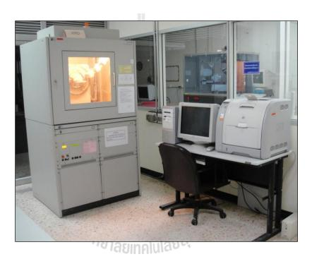
Figure 3.10 X-ray diffractometer (Bruker D5005).
