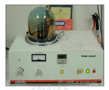
Figure 3.13 Ion sputtering machine JEOL JCF-1100E.
