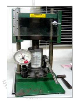
Figure 3.5 Hydraulic presser CARVER hydraulic unit model #3912.
