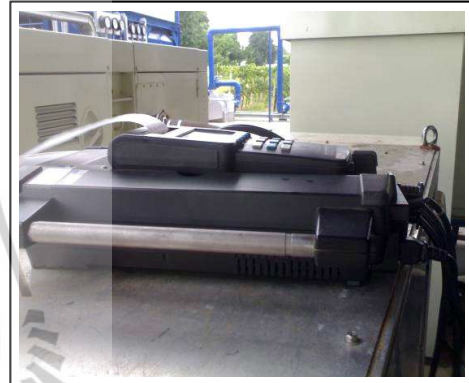
ง. Flue Gas Analyzer
