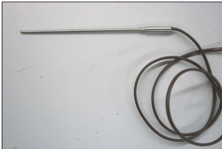
Figure 3.31 Temperature sensor (Thermocouple).
