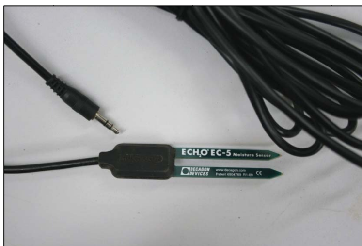
Figure 3.32 Moisture sensor (EC-5).
