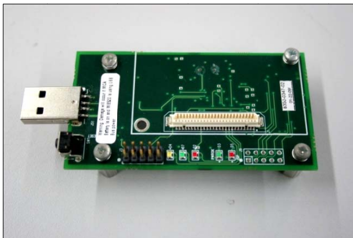
Figure 3.28 MIB520CB (USB interface board).
