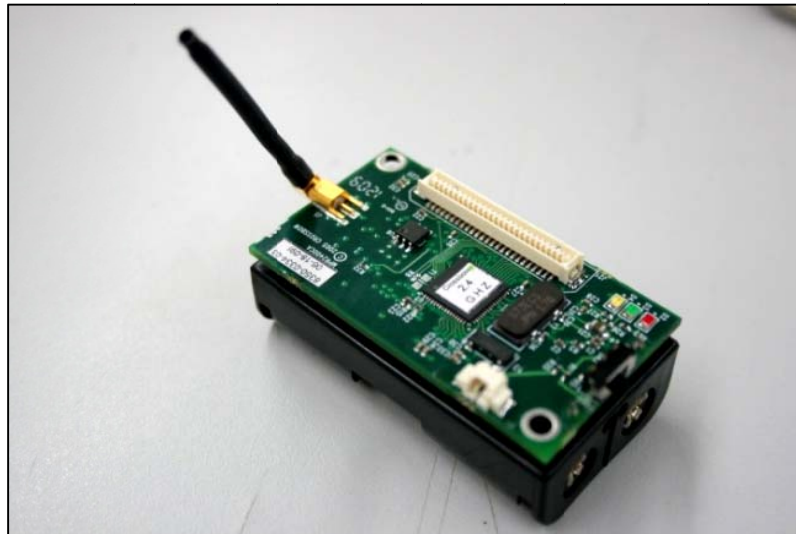
Figure 3.29 Sensor node model MPR2400 or MicaZ.
