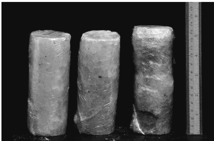
Figure 4.2 Examples of post-test specimens from the uniaxial cyclic loading test.
