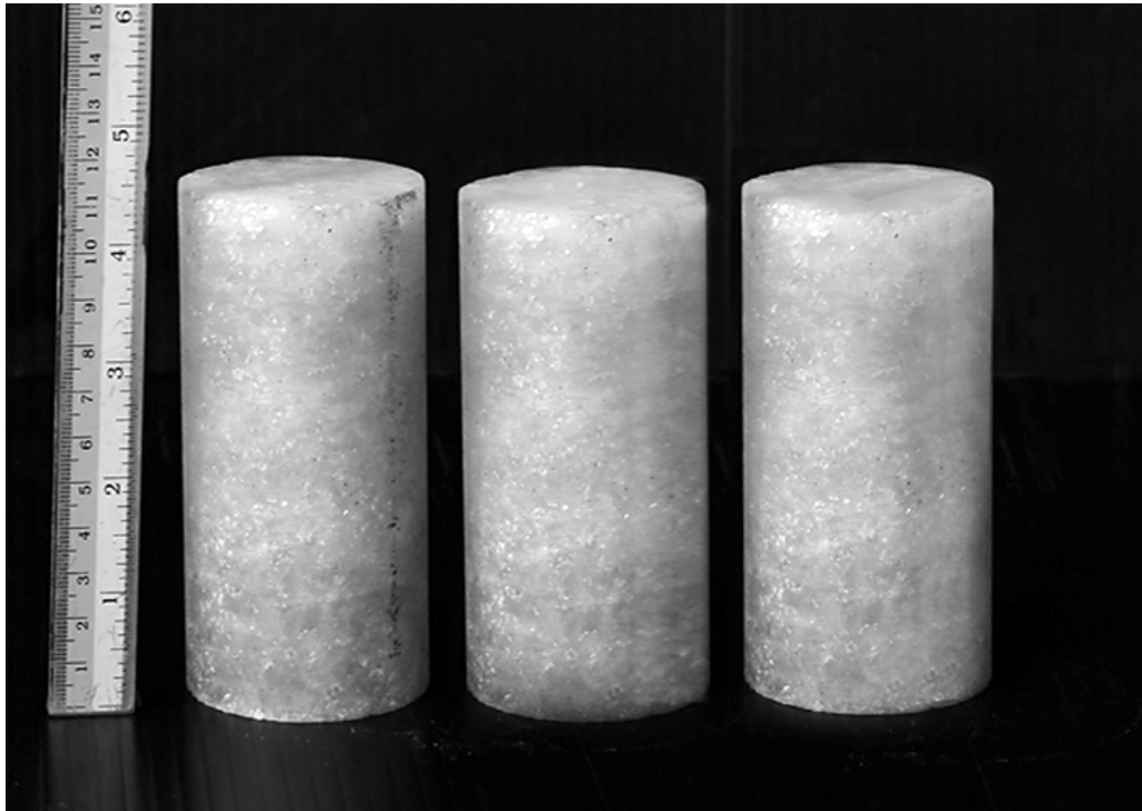
Figure 3.3 Some rock salt specimens prepared for triaxial creep tests L/D = 2.0
