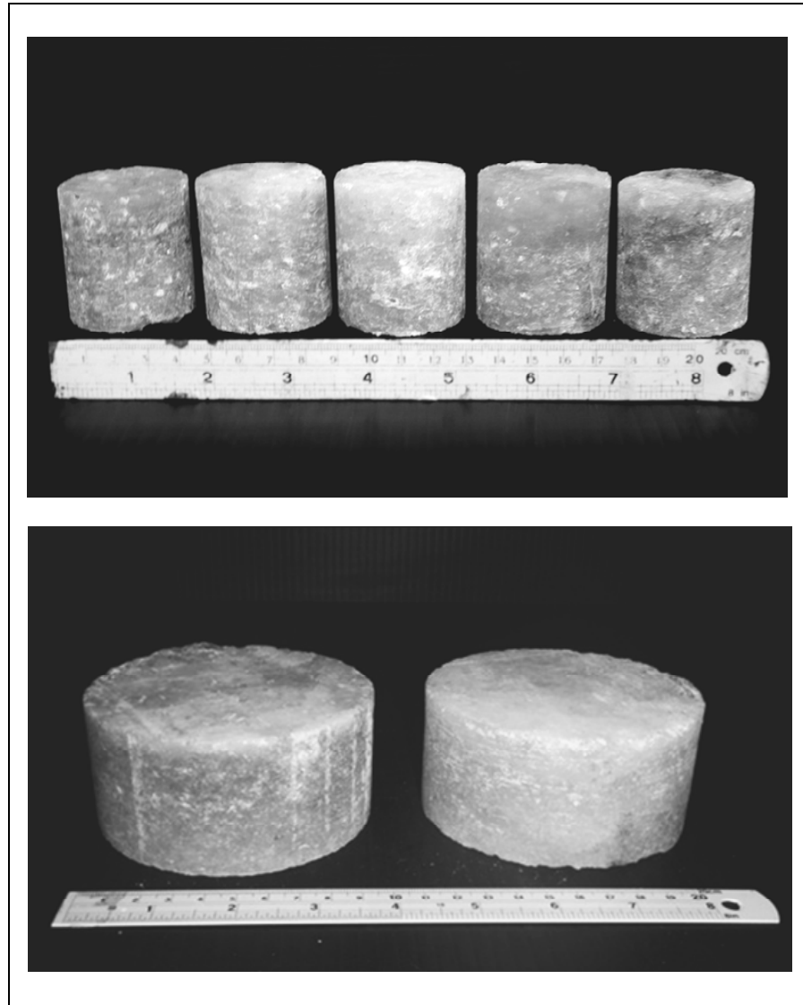
Figure 3.4 Some rock salt specimens prepared for MPL creep tests with D/d = 2 (top) and D/d = 4 (bottom).
