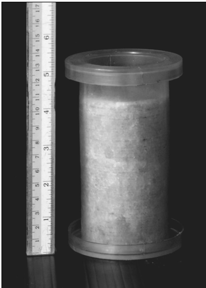
Figure 4.22 Some specimen post-test of triaxial creep tests.
