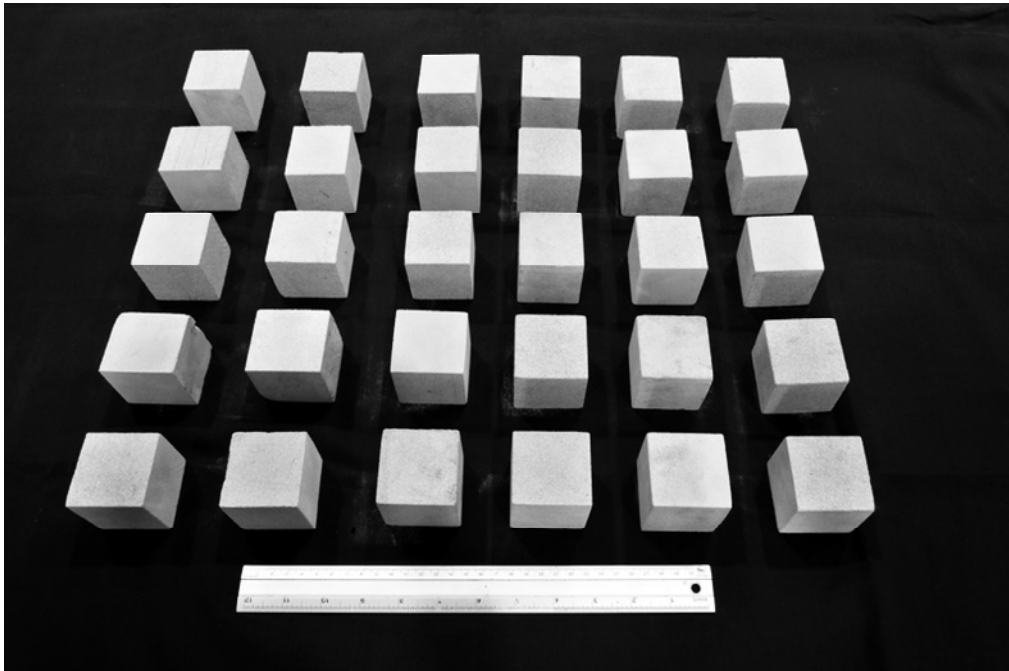
Figure 3.1 Some PW sandstone specimens prepared for polyaxial compression testing.
